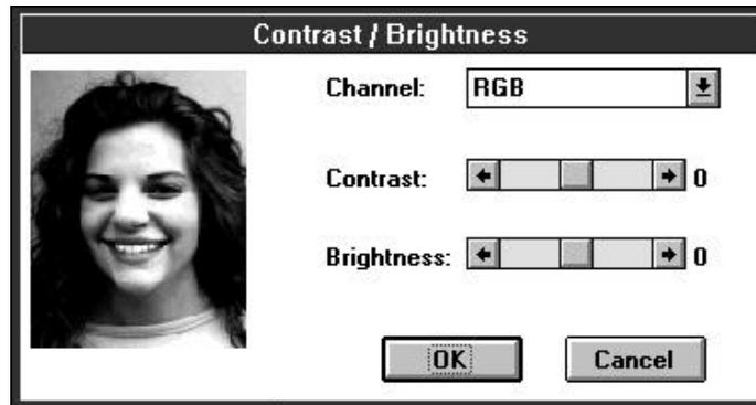
Use these menu items to increase the contrast and brightness of the selected image. Contrast will make dark parts of an image darker and will make light colors lighter. Brightness will make the entire image lighter. Use the slider controls to change the contrast and brightness on the preview image which is displayed. Then select OK to apply those changes to the image. You can use
