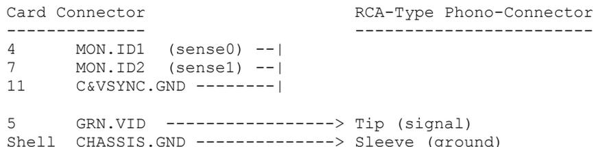
By grounding pin 4 and pin 7 to pin 11, the Macintosh Quadra computers are told that an NTSC monitor is attached. The actual black-and-white video signal is on pin 5 and connects to the center (Tip) of the phono-plug. The shell of the card connector connects to the sleeve of the phono-plug.
