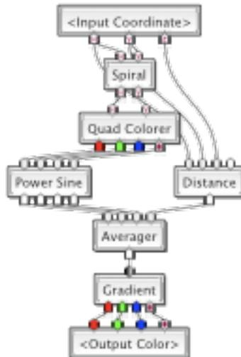
In this example, the starting input coordinate (the location on the image) are fed down in to a “Spiral” and a “Distance” node, the “Spiral” goes on to a “Quad Colorer” which feeds a “Power Sine”, and something called “Averager” combines them all together, and then it goes to “Gradient” which finally connects to the “<Output Color>”. You can think of this diagram as the “DNA” of the image. If one were to write this out, it might look something like this:
