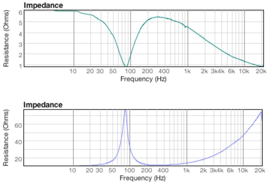
*The graph on the top demonstrates an upside-down impedance measurement, while the graph on the bottom shows one that's correctly oriented.*
