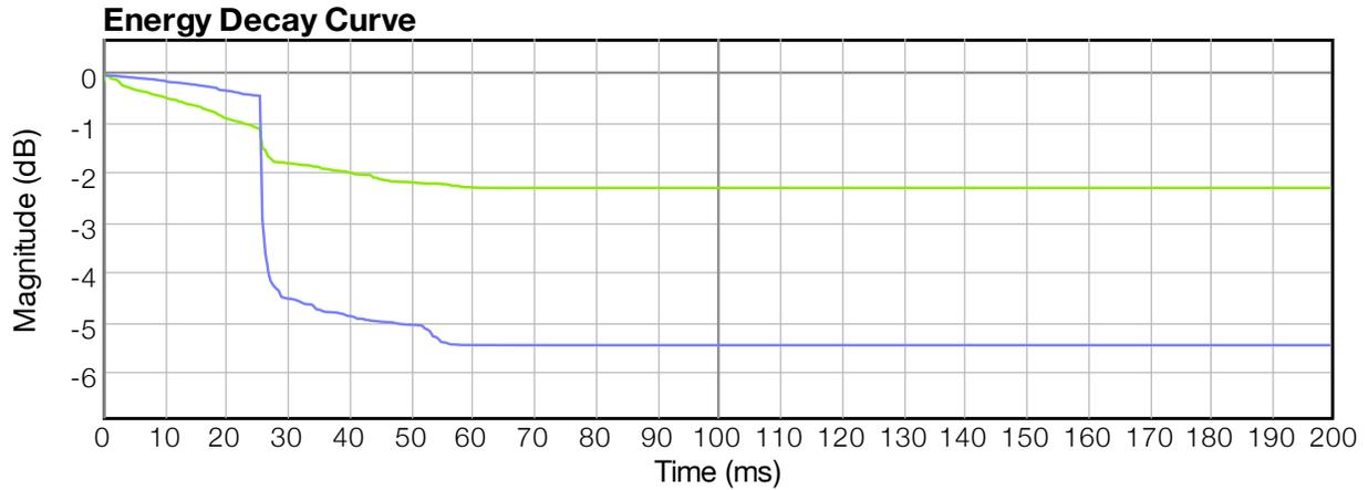
*In the graph above, the green curve represents a measurement done at a low volume with 1 synchronous average. The blue curve represents the exact same settings, except with 16 synchronous averages. Note how the theoretical increase of 12dB was not achieved.*
