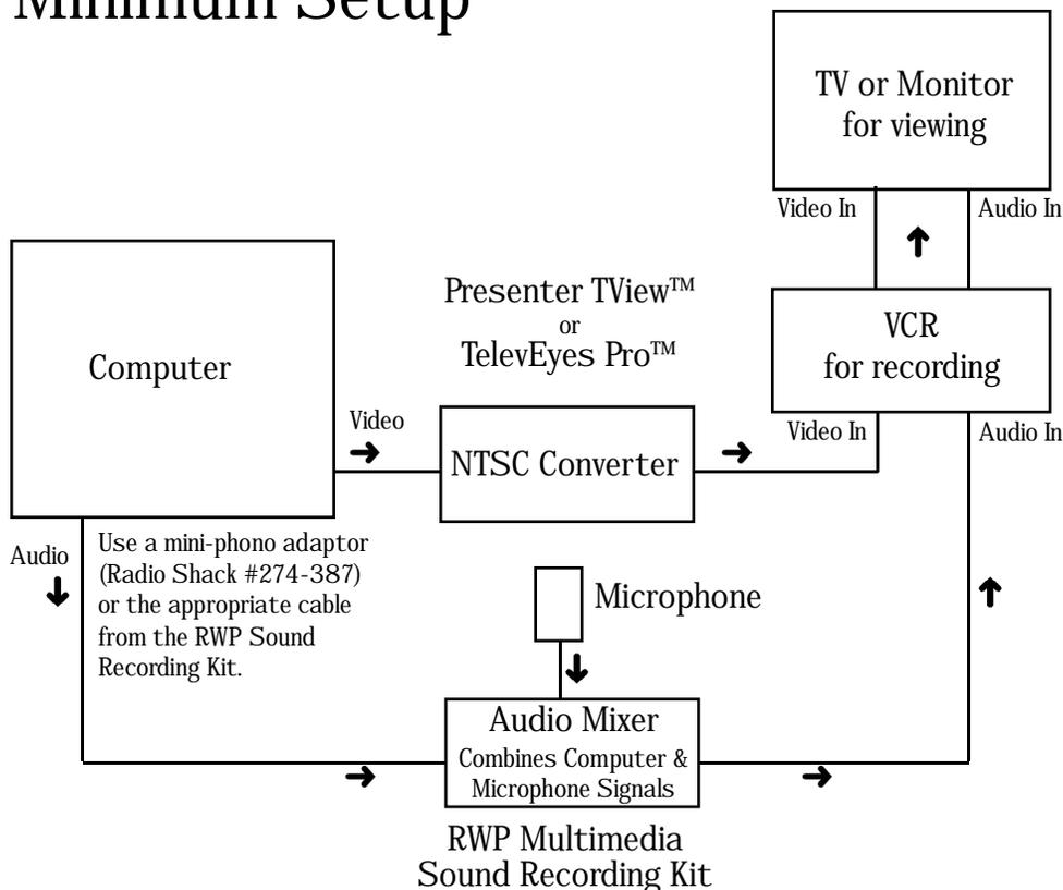
This is the minimum setup you'll need to record computer presentations on a video cassette recorder (VCR). It provides for the video signal to be sent from the computer to the TV/monitor; and, provides for the audio signal to be sent from both the computer and a microphone.
