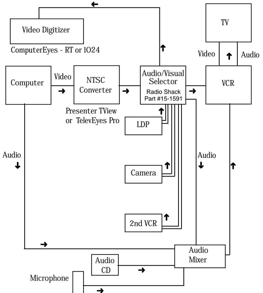
This setup provides for recording presentations (both video and audio portions), and for digitizing images from various video sources. A video source can be any kind of equipment that produces a video signal. In this diagram we show a laserdisc player, video camera and a second VCR as sources for digitizing images on the computer. The Audio/Visual Selector makes it very convenient for switching between different sources of both audio and video signals.
