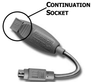
NB. Connecting devices to the ADB port when your Mac is not shutdown risks damaging both the port and the devices.
