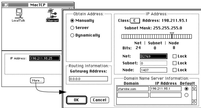
Figure 4 Checking the MacTCP Control Panel configuration
