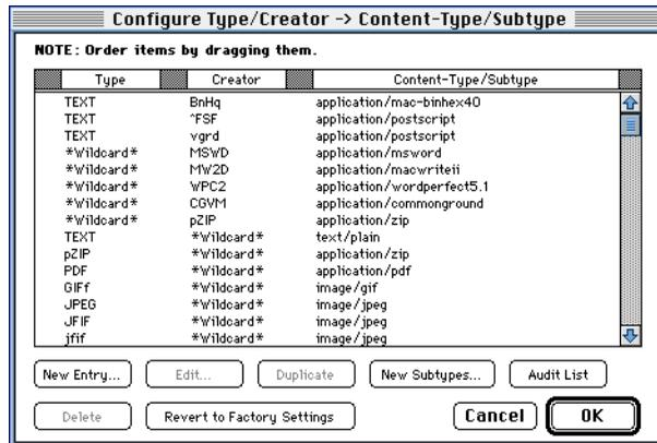
Figure 36 Mac type/creator to MIME Content-type/subtype mapping
