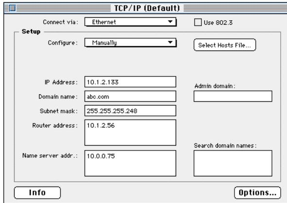
Figure 3 Checking the Open Transport configuration
