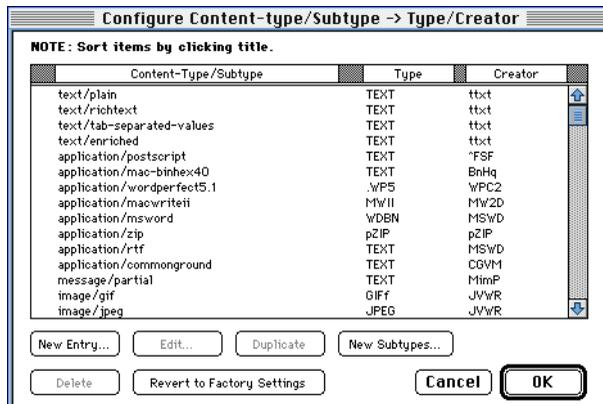
Figure 42 MIME Content-type/subtype mapping to Mac type/creator
