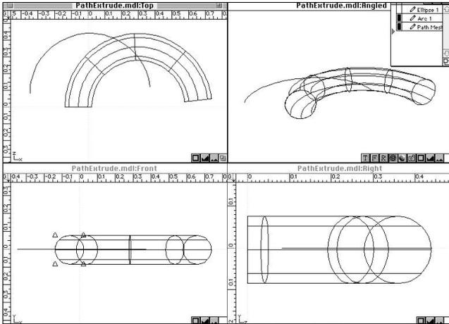
The selected shape(s) will be placed at the end of the path, and made perpendicular to the path, and then “extruded” along the path and transformed in a linear fashion according to the ending width and height that was specified. A new, surfaced object will be created along that extrusion. The original objects are saved separately and “turned-off” in the Group palette unless otherwise specified in Preferences. They can be restored at anytime.
