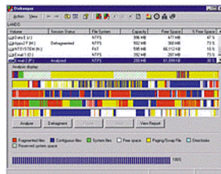
Figure 1: Graphic analysis: The red areas represent fragmented files and the white show fragmented free space. Note that system files (green) and Paging File (yellow) are seriously affected. With a disk in this condition, performance is slowed markedly. The longer a user waits to defragment his or her disk volumes, the worse the computer runs.
