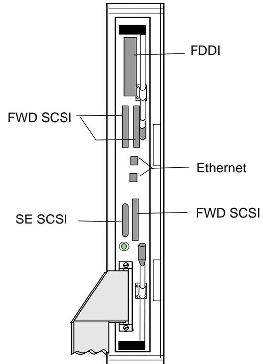
Figure 7 KFTHA Module with Four Channels
