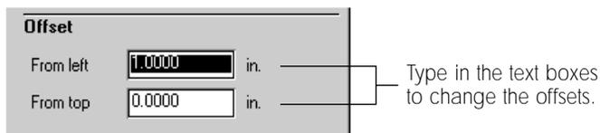
You can enter a new offset in any measurement unit you like (inches, centimeters, points, or picas); Informed Designer performs the appropriate unit conversion for you. After entering a new offset, press Tab (or Shift-Tab) to update the drawing setup on the dialog box.
