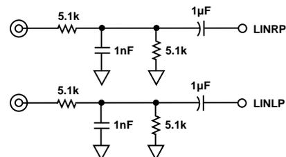
Figure 18. AD1843 2 V rms Single-Ended Line-Level Input Circuit
