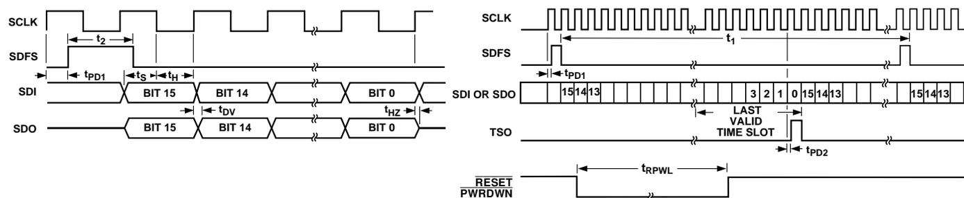
Figure 1. Timing Diagrams
