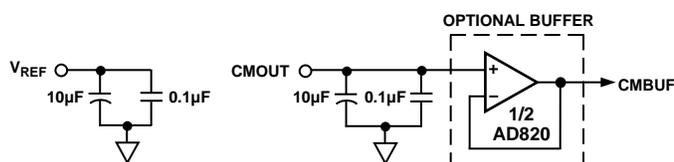
Figure 27. AD1843 Voltage Reference Bypassing
