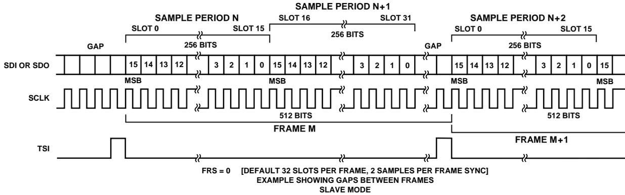
Figure 9a. FRS = 0, Slave Mode Timing
