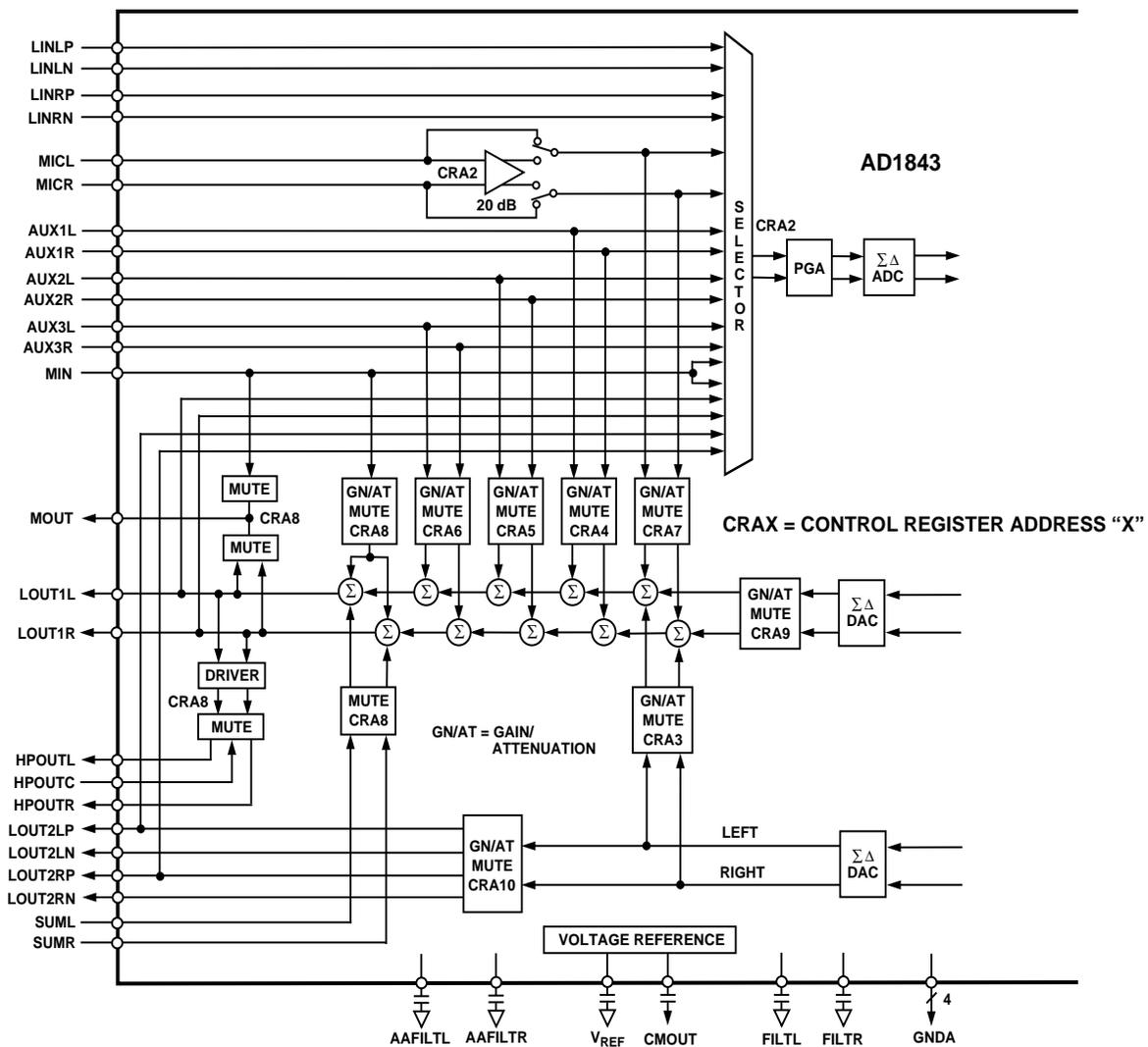
Figure 12. AD1843 Control Registers Associated with Block Diagram
