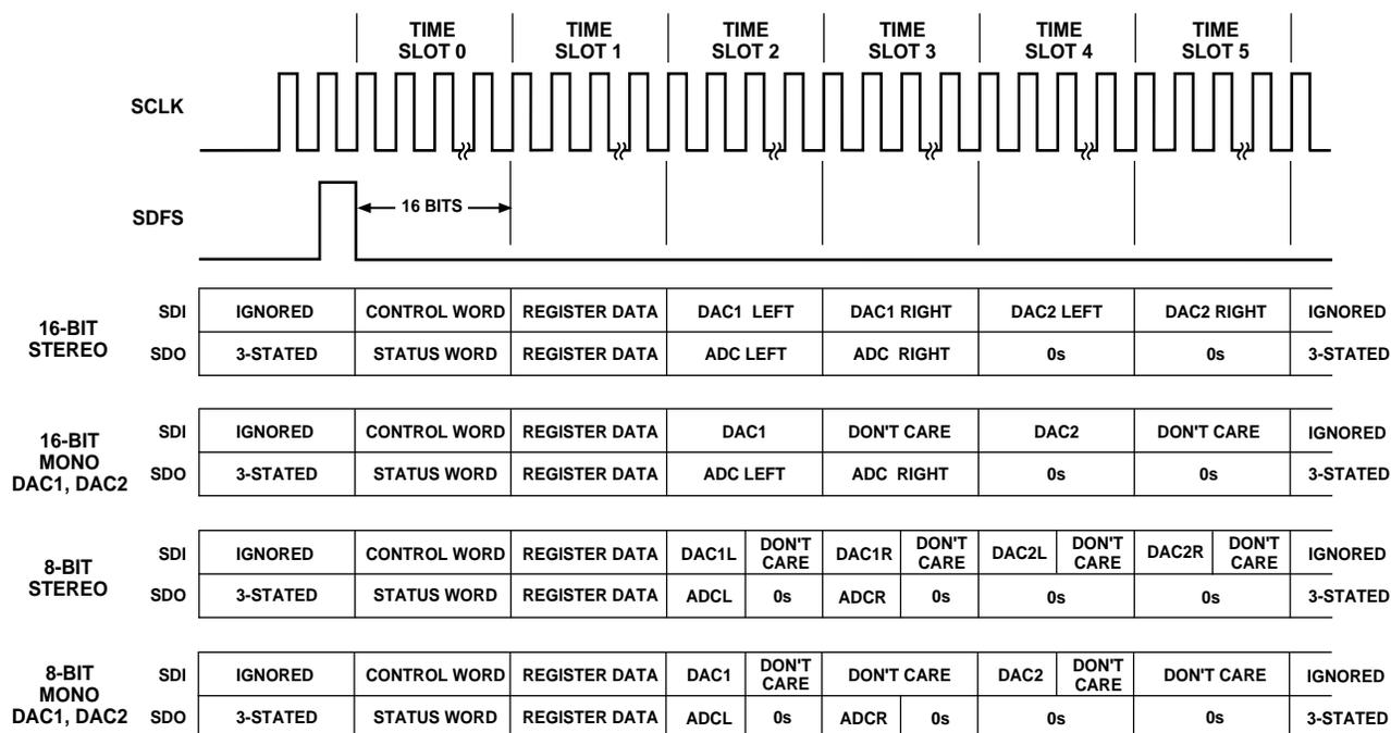
THE DIAGRAM ABOVE IS INTENDED TO BE ILLUSTRATIVE OF THE MORE COMMONLY USED CONFIGURATIONS. ADC LEFT, ADC RIGHT, DAC1 AND DAC2 CAN BE INDIVIDUALLY ASSIGNED TO 8-BIT OR 16-BIT SAMPLE WIDTH, AND DAC1 AND DAC2 CAN BE INDIVIDUALLY ASSIGNED TO STEREO OR MONO MODE. EACH AD1843 CONSUMES 6 TDM SLOTS (REQUIRING 96 SCLK PERIODS), LEAVING 10 TDM SLOTS UNUSED IN A 16 SLOT FRAME.
