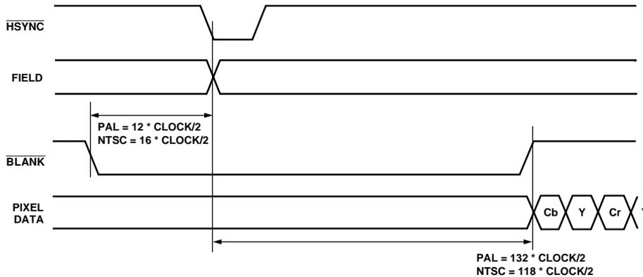
Figure 19. Timing Mode 1 Odd/Even Field Transitions
