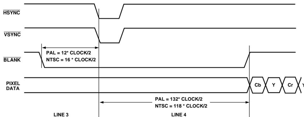
Figure 22. Timing Mode 2 Even-to-Odd Field Transition
