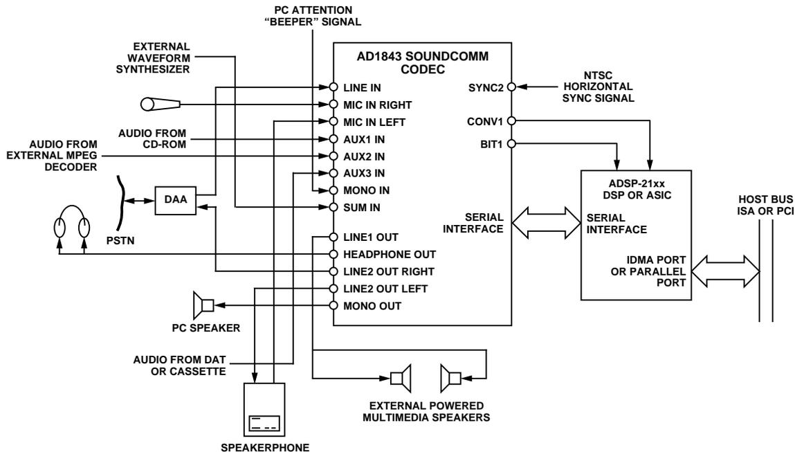
Figure 6. Typical Configurations
