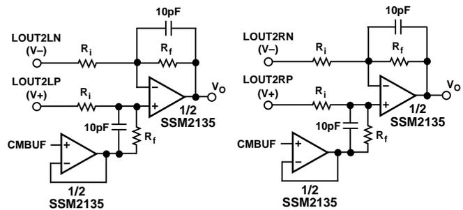
Figure 24. AD1843 Differential-to-Single-Ended Converter Line Output Connections
