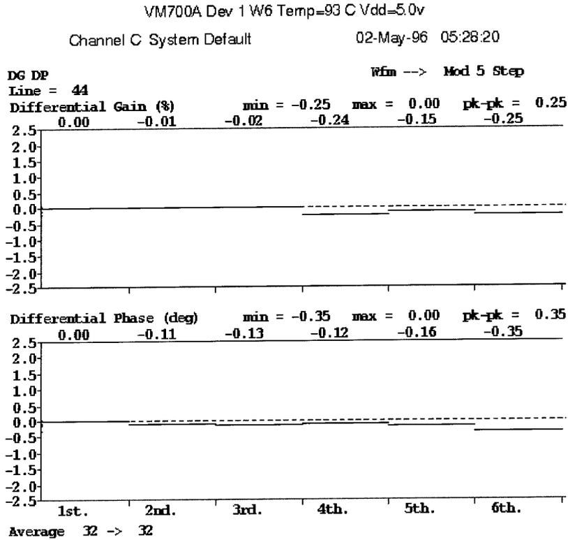
Figure 61. Differential Phase and Gain Measurements (PAL)
