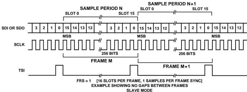
Figure 10b. FRS = 1, Slave Mode Timing
