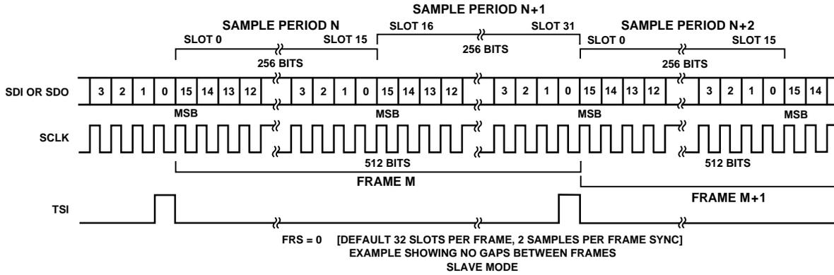
Figure 9b. FRS = 0, Slave Mode Timing
