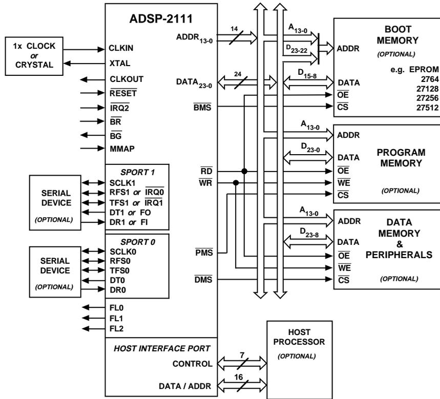
THE TWO MSBs OF THE DATA BUS (D<sub>23-22</sub>) ARE USED TO SUPPLY THE TWO MSBs OF THE BOOT MEMORY EPROM ADDRESS. THIS IS ONLY REQUIRED FOR THE 27256 AND 27512.
