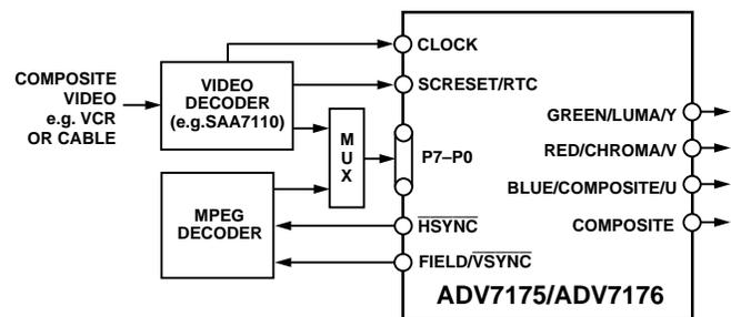
Figure 12. RTC Connections
