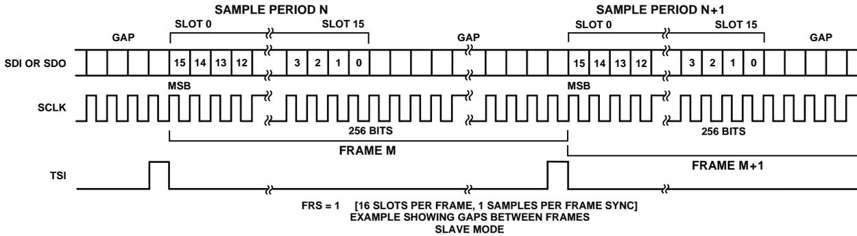
Figure 10a. FRS = 1, Slave Mode Timing
