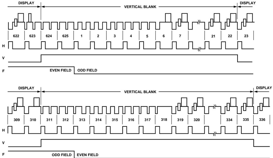
Figure 15. Timing Mode 0 (PAL Master Mode)
