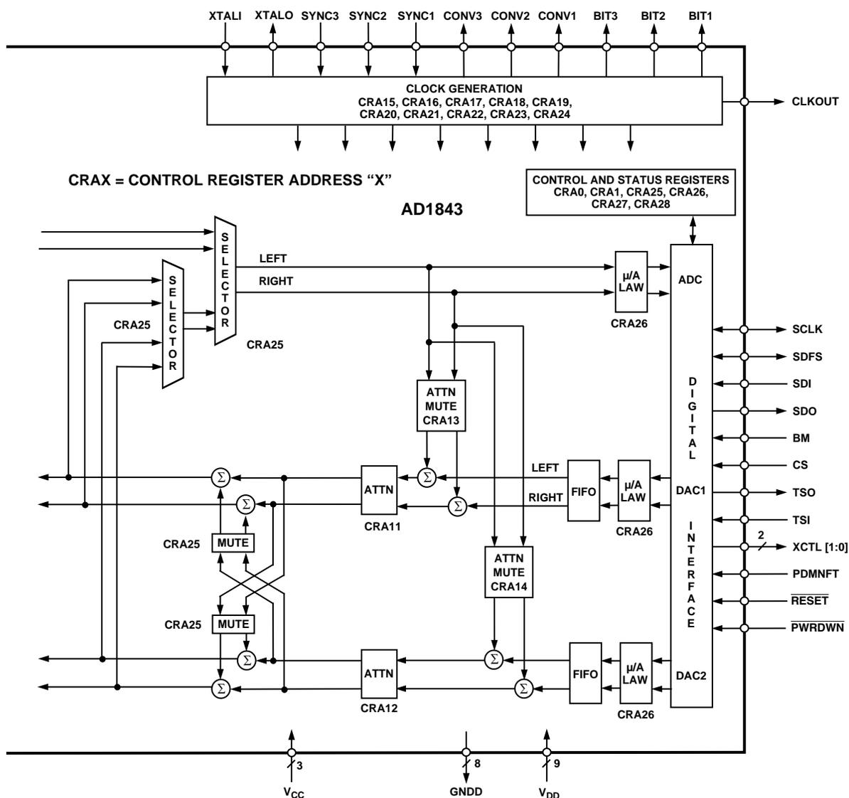
Figure 13. AD1843 Control Registers Associated with Block Diagram
