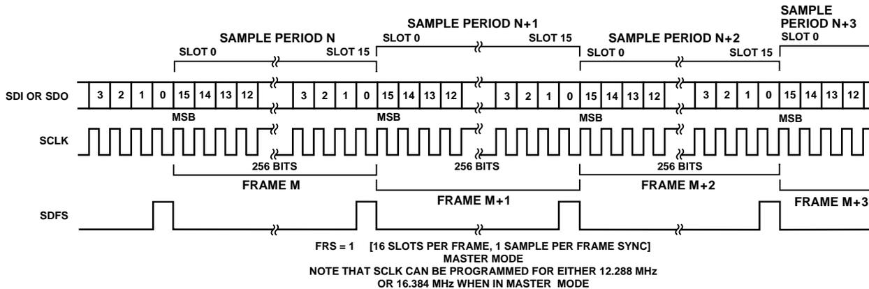
Figure 8. FRS = 1, Master Mode Timing
