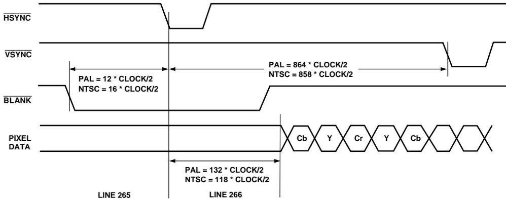
Figure 23. Timing Mode 2 Odd-to-Even Field Transition
