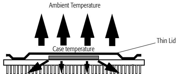
**Figure 93. Processor Heat Dissipation Path**
