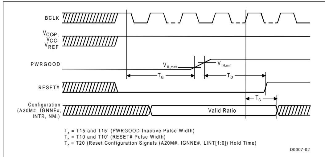
Figure 11. Test Timings (TAP Connection)
