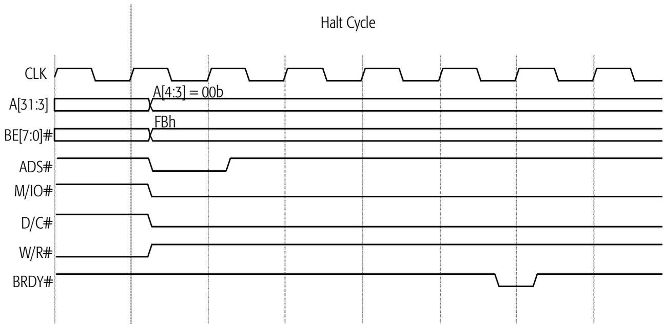
Figure 62. Basic Special Bus Cycle (Halt Cycle)
