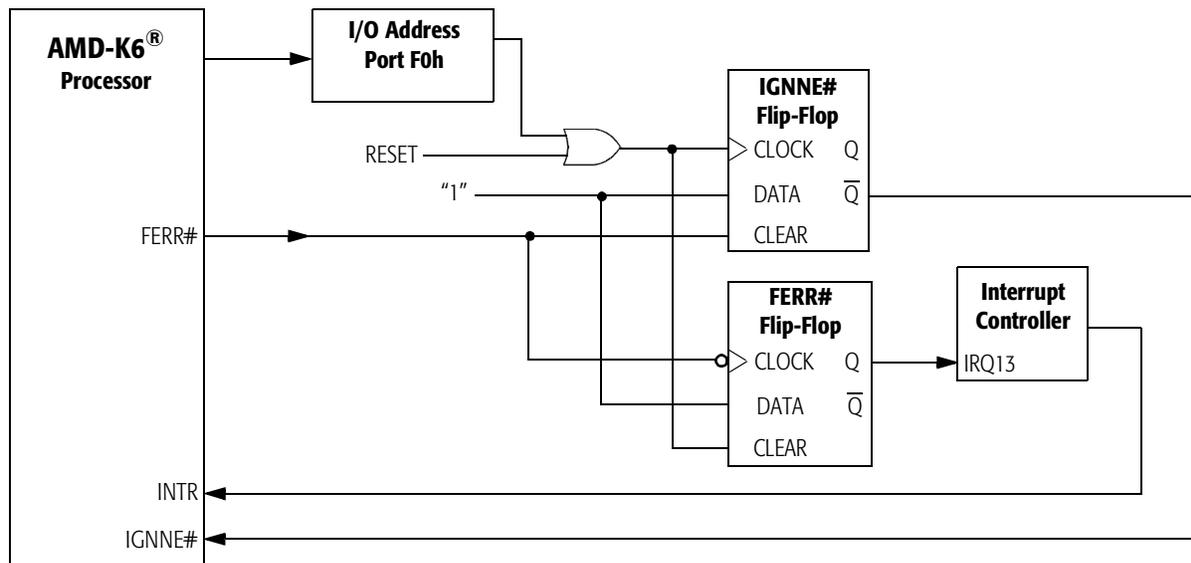
**Figure 71. External Logic for Supporting Floating-Point Exceptions**
