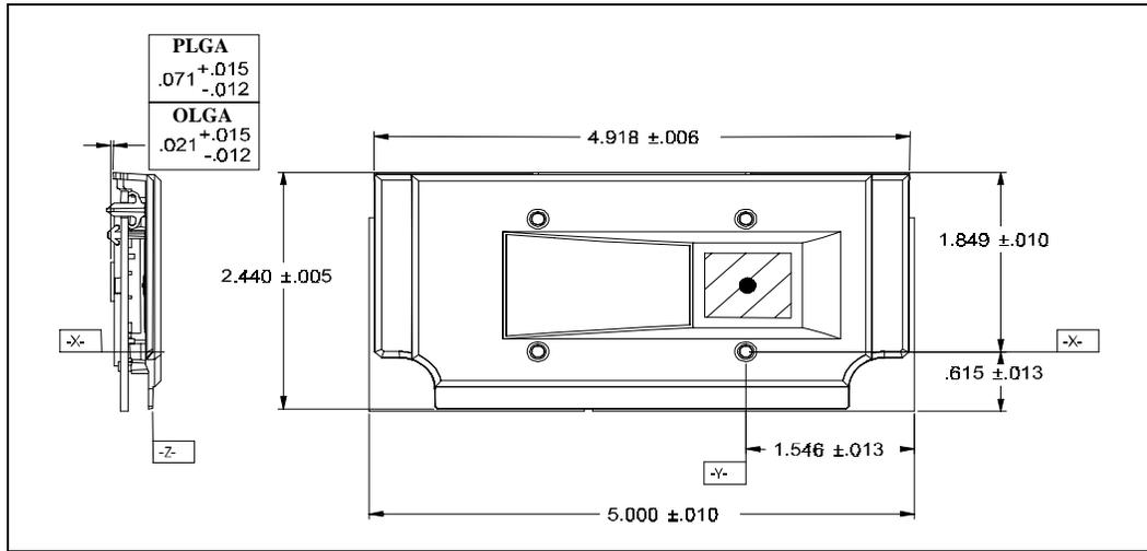
Figure 32. Pentium® II Processor Assembly (S.E.C.C.2 Package)—Heat Sink Attach Boss Section
