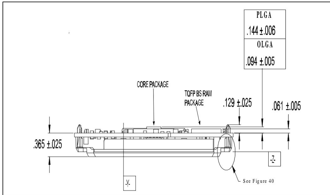
Figure 34. Detail View of Cover in the Vicinity of the Substrate Attach Features
