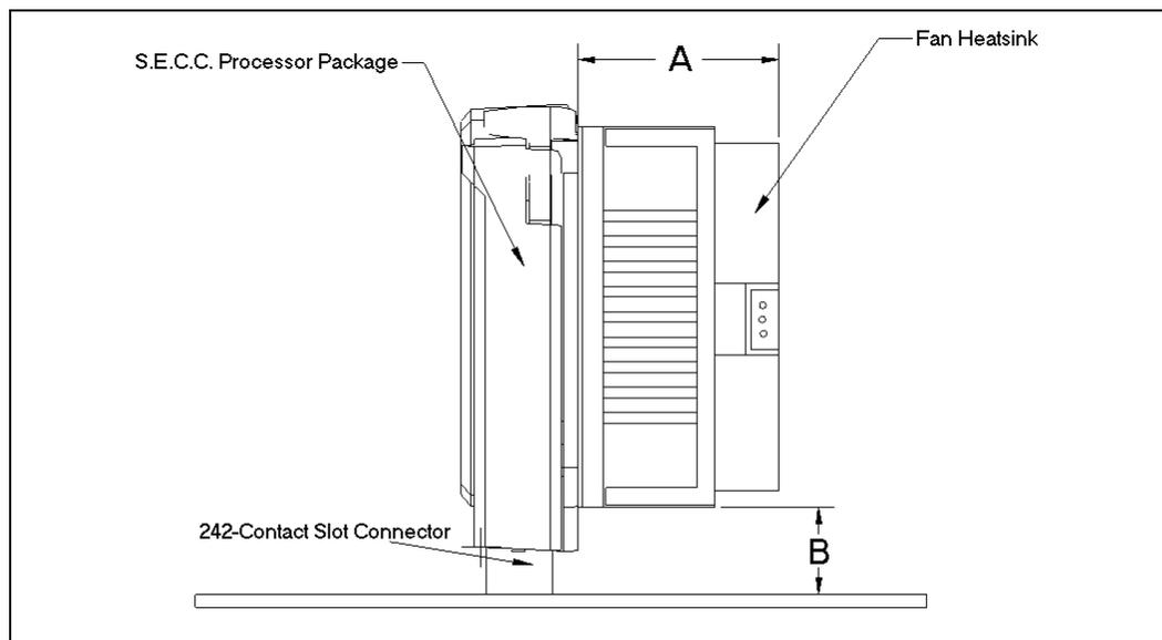
Figure 40. Front View Space Requirements for the Boxed Processor with S.E.C.C. Packaging
