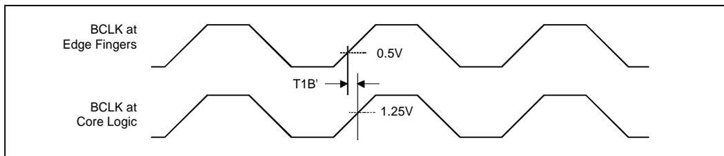
**Figure 3. BCLK\*, PICCLK, and TCK Generic Clock Waveform**
