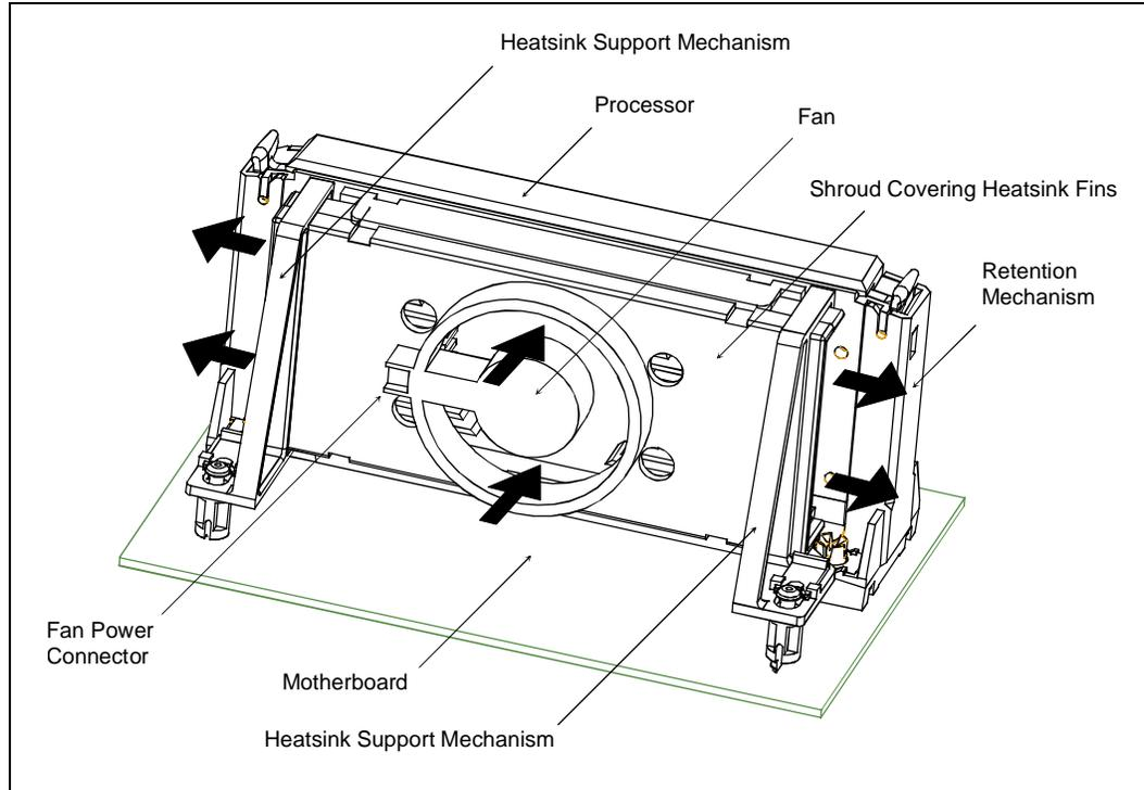
**Figure 38. Boxed Pentium® II Processor in the S.E.C.C.2 Packaging (Fan Power Cable Not Shown)**
