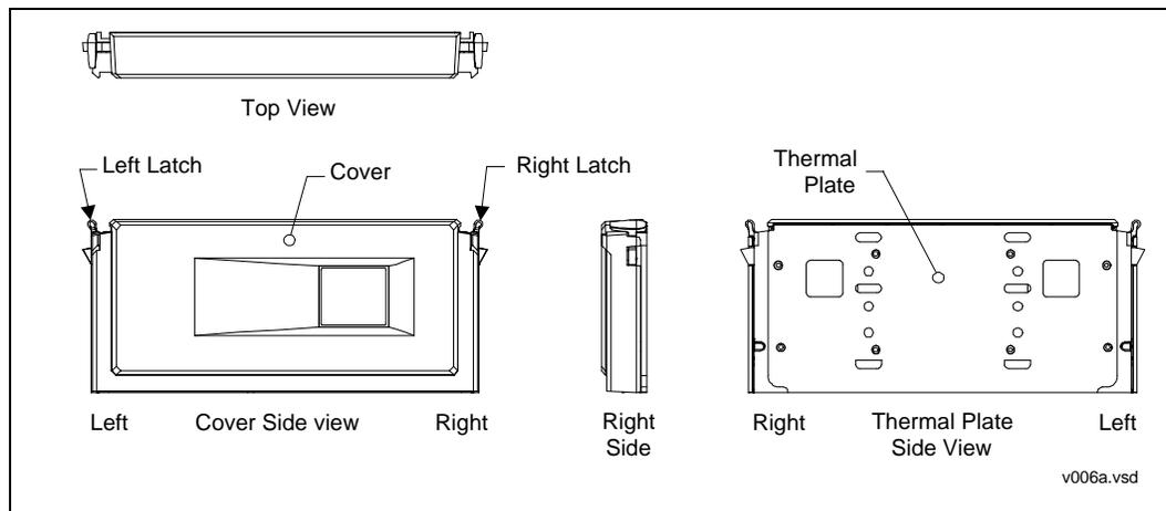
Figure 19. Pentium® II Processor (S.E.C.C. Package)—Extended Thermal Plate Side Dimensions
