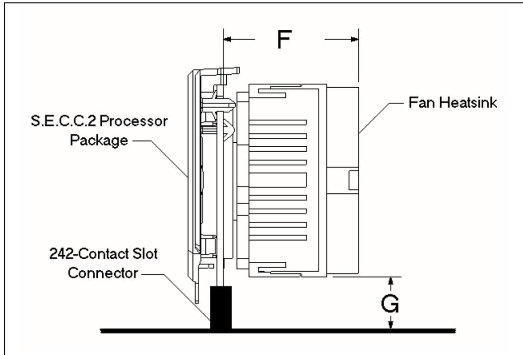
Figure 42. Front View Space Requirements for the Boxed Processor with S.E.C.C.2 Packaging
