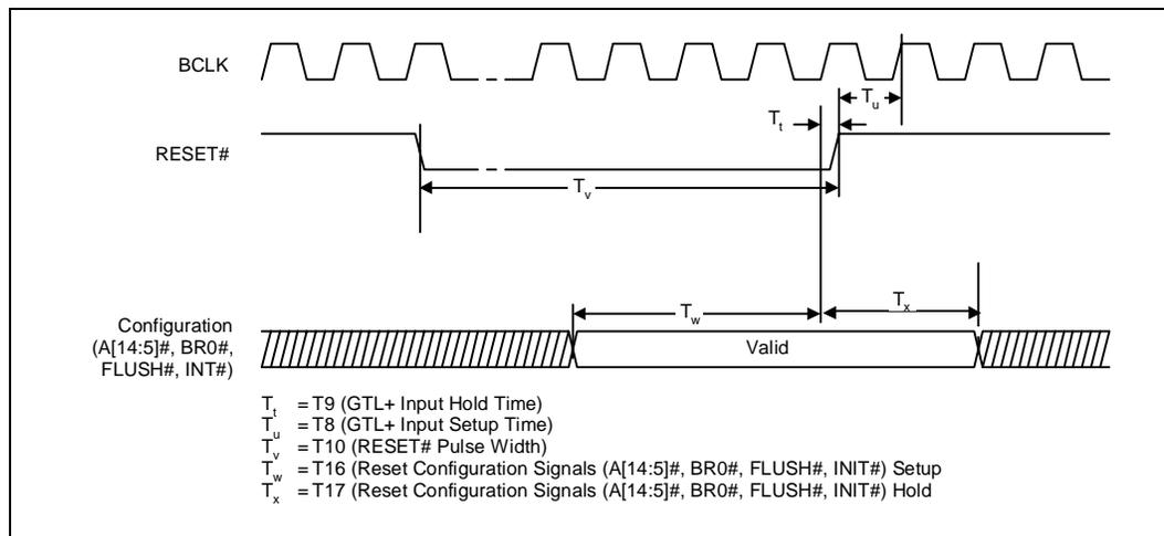
Figure 7. Power-On Reset and Configuration Timings
