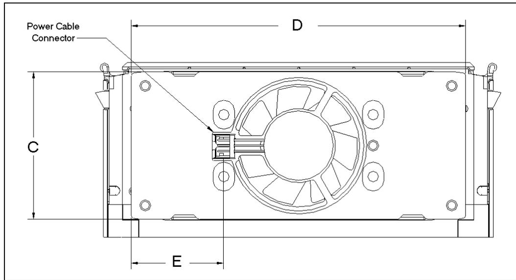
Figure 41. Side View Space Requirements for the Boxed Processor with S.E.C.C.2 Packaging
