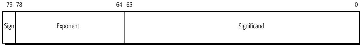
Figure 11. Floating-Point Register
