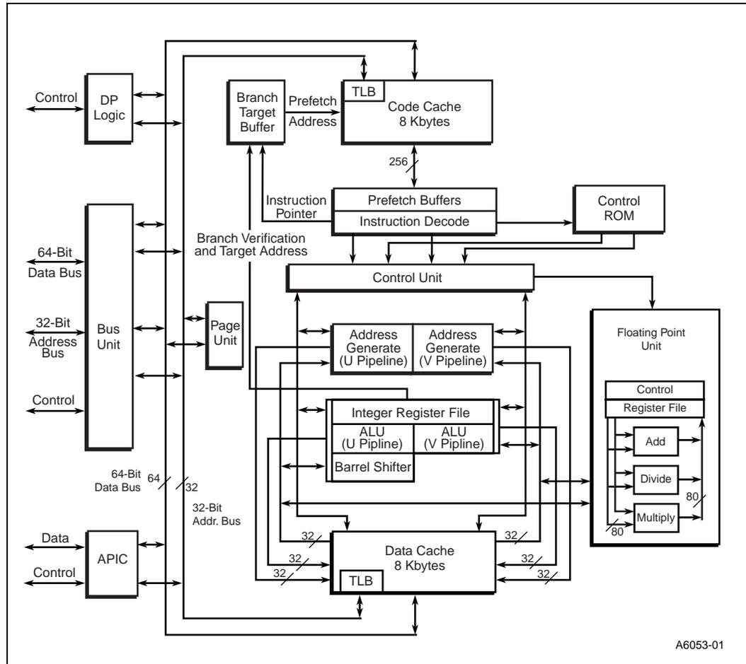
The block diagram shows the two instruction pipelines, the “u” pipe and the “v” pipe. The u-pipe can execute all integer and floating-point instructions. The v-pipe can execute simple integer instructions and the FXCH floating-point instructions.
