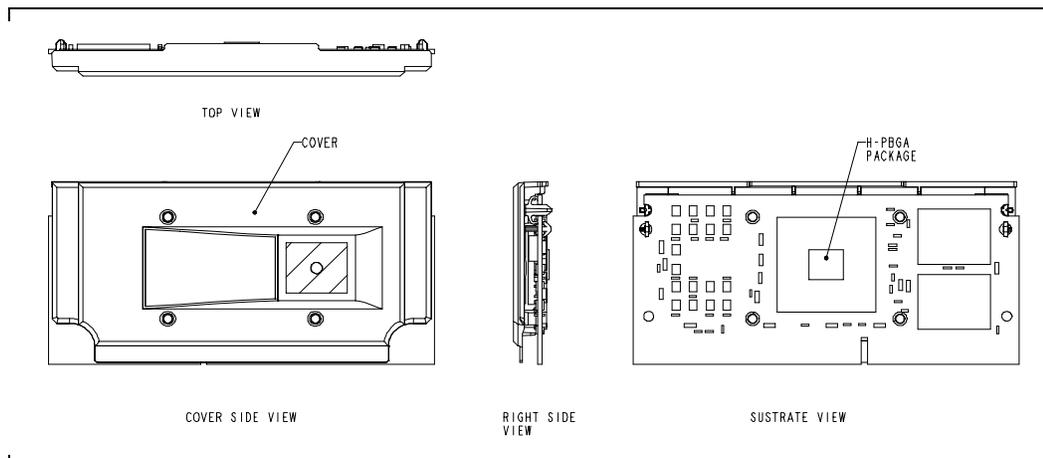
Figure 29. Pentium® II Processor (S.E.C.C.2 Package) Top and Side Views—PLGA Processor Core
