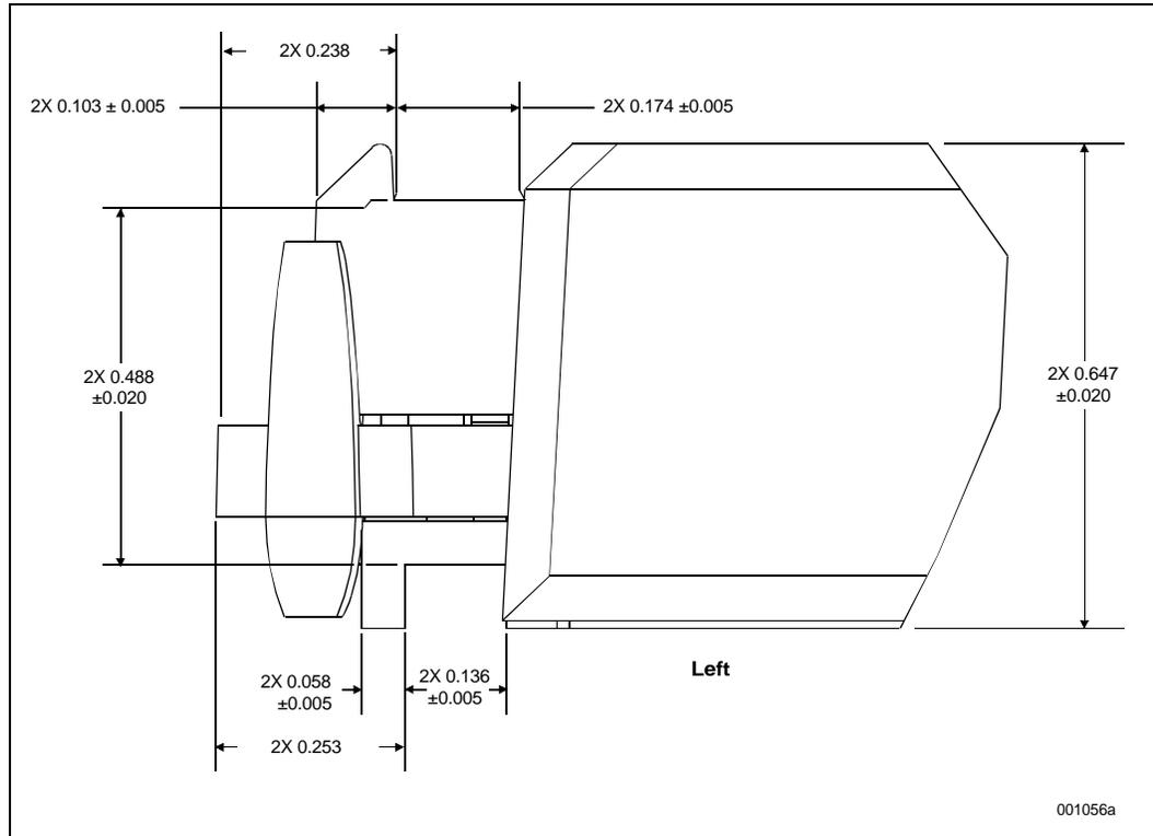
**Figure 22. Pentium® II Processor (S.E.C.C. Package)—Latch Arm, Extended Thermal Plate, and Cover Detail Dimensions (Reference Dimensions Only)**
