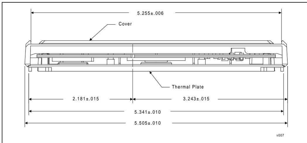
Figure 21. Pentium® II Processor (S.E.C.C. Package)—Latch Arm, Extended Thermal Plate Lug, and Cover Lug Dimensions
