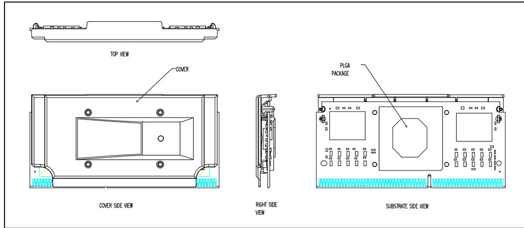
Figure 30. Pentium® II Processor Assembly (S.E.C.C.2 Package)—Primary View
