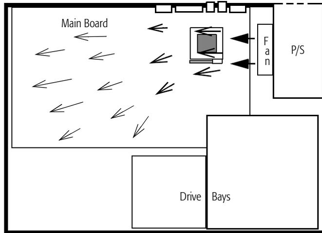
**Figure 98. Airflow Path in an ATX Form-Factor System**
