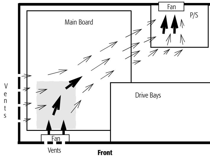
**Figure 97. Airflow Path in a Dual-fan System**
