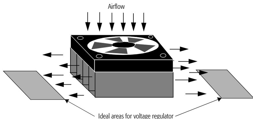
**Figure 96. Airflow for a Heatsink with Fan**
