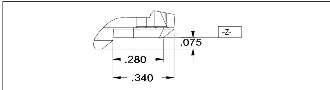
Figure 35. Pentium® II Processor Substrate (S.E.C.C.2 Package), Edge Finger Contact Dimensions
