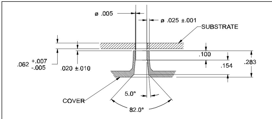
Figure 33. Pentium® II Processor Assembly (S.E.C.C.2 Package), Side View—OLGA Substrate Shown
