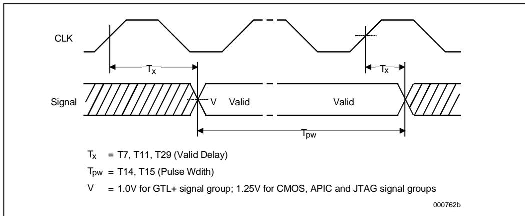
**Figure 8. System Bus Setup and Hold Timings**
