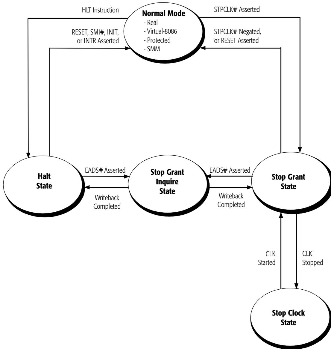
Figure 78. Clock Control State Transitions
