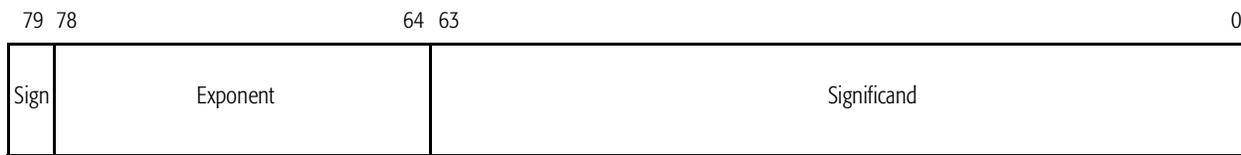
Figure 10. Floating-Point Register
