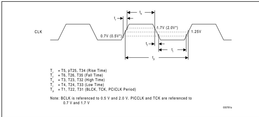
**Figure 7. System Bus Valid Delay Timings**
