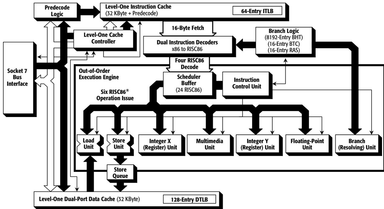
Figure 1. AMD-K6<sup>®</sup> Processor Block Diagram
