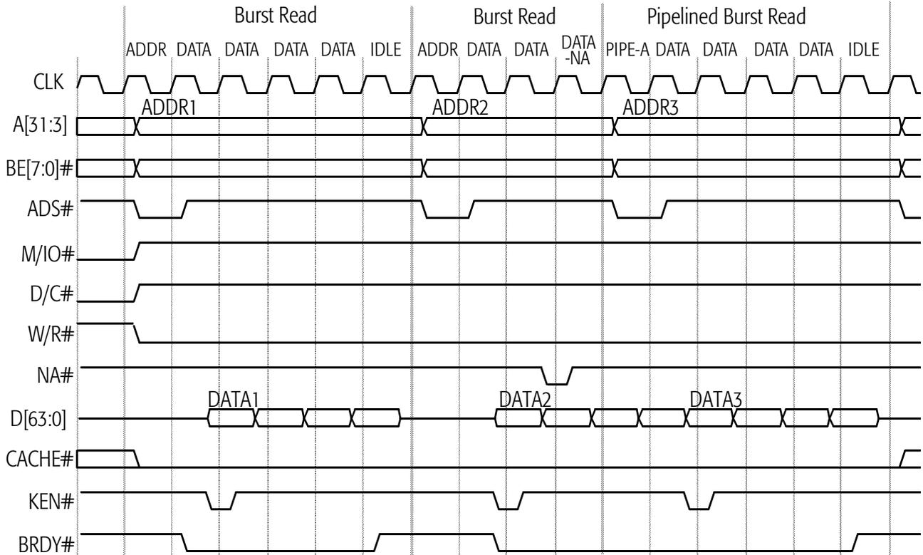
**Figure 47. Burst Reads and Pipelined Burst Reads**
