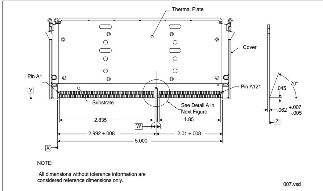
Figure 26. Pentium® II Processor Substrate (S.E.C.C. Package)—Edge Finger Contact Dimensions, Detail A
