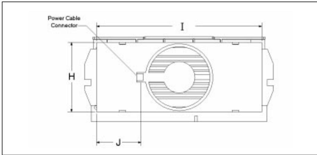
Figure 43. Top View Air Space Requirements for the Boxed Processor
