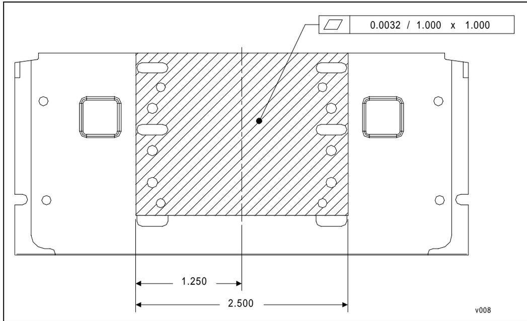
**Figure 25. Pentium® II Processor Substrate (S.E.C.C. Package)—Edge Finger Contact Dimensions**
