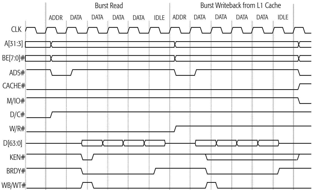
**Figure 48. Burst Writeback due to Cache-Line Replacement**
