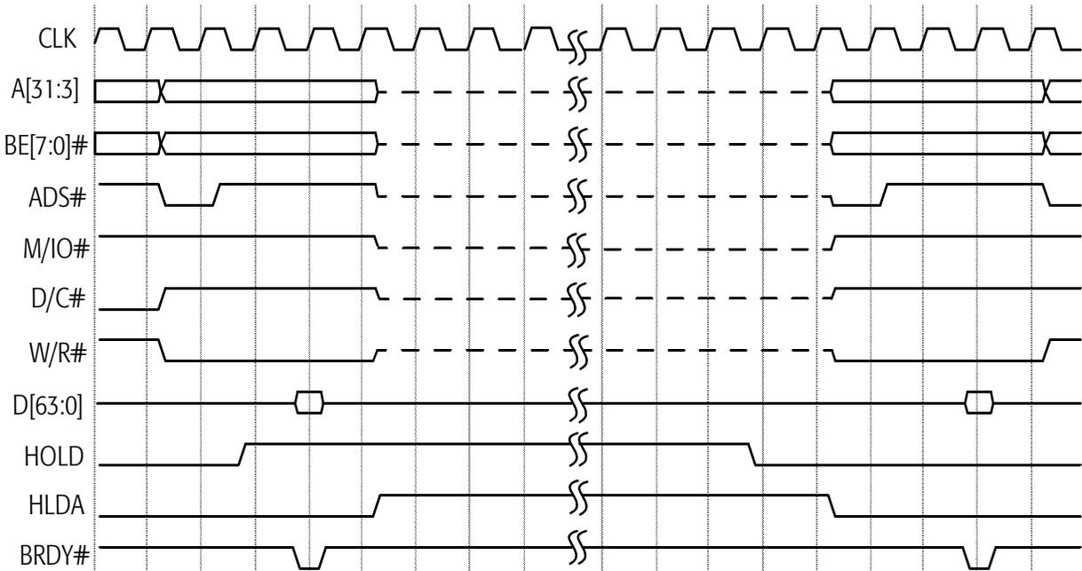
Figure 51. Basic HOLD/HLDA Operation
