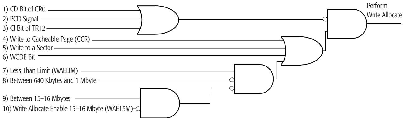
**Figure 70. Write Allocate Logic Mechanisms and Conditions**
