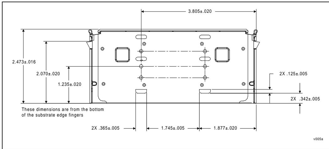
Figure 20. Pentium® II Processor (S.E.C.C. Package)—Bottom View Dimensions
