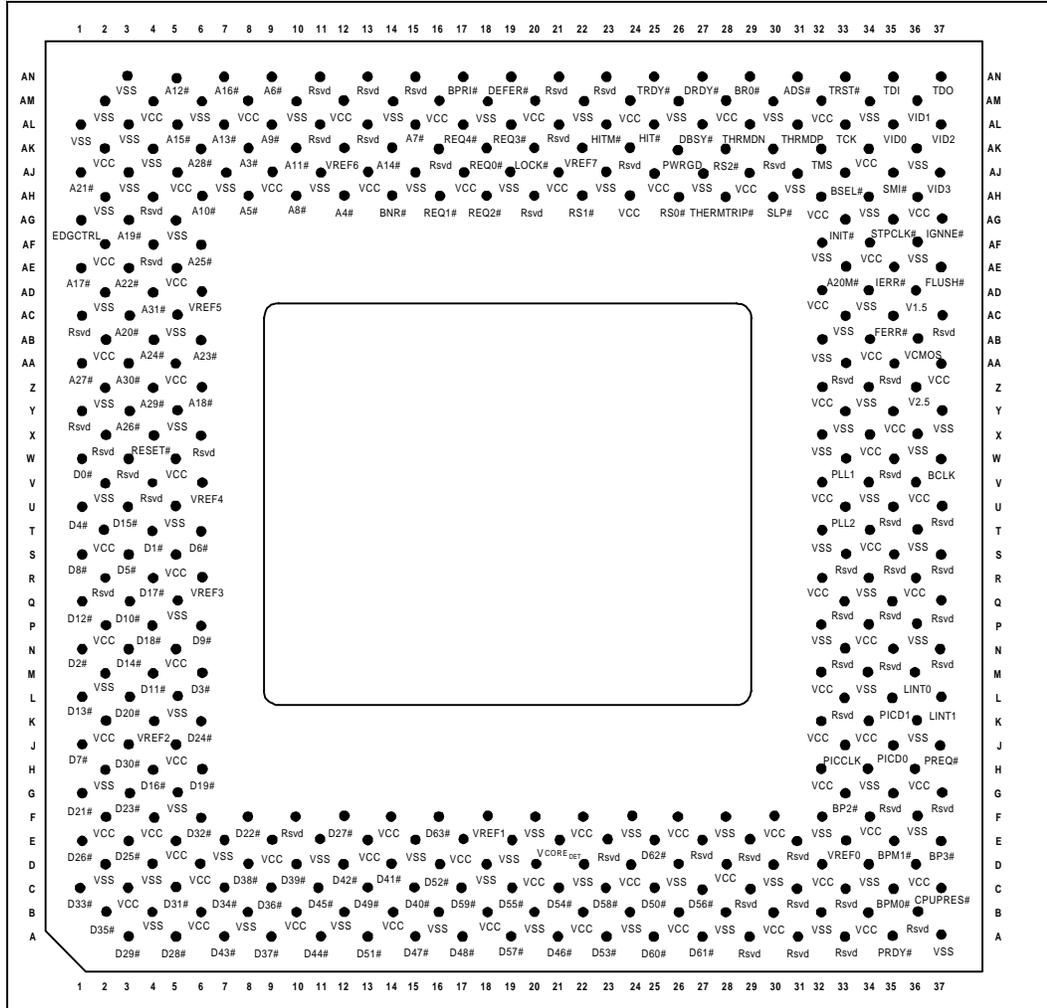
**Table 36. PPGA Package Signal Listing in Order by Pin Number (Sheet 1 of 6)**
