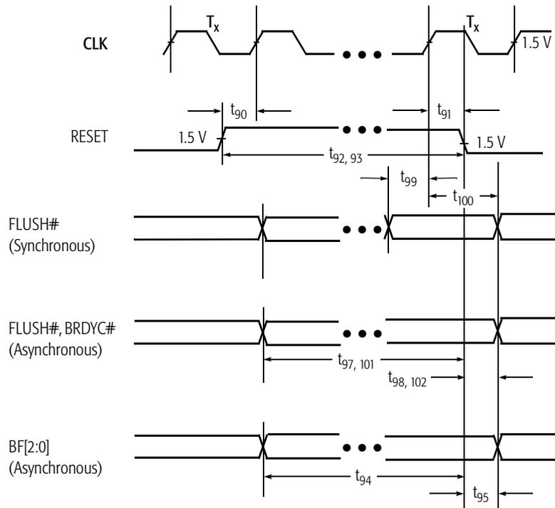
Figure 87. Reset and Configuration Timing
