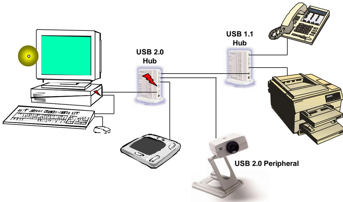
**Figure 2. Future USB 2.0 System Configuration**
