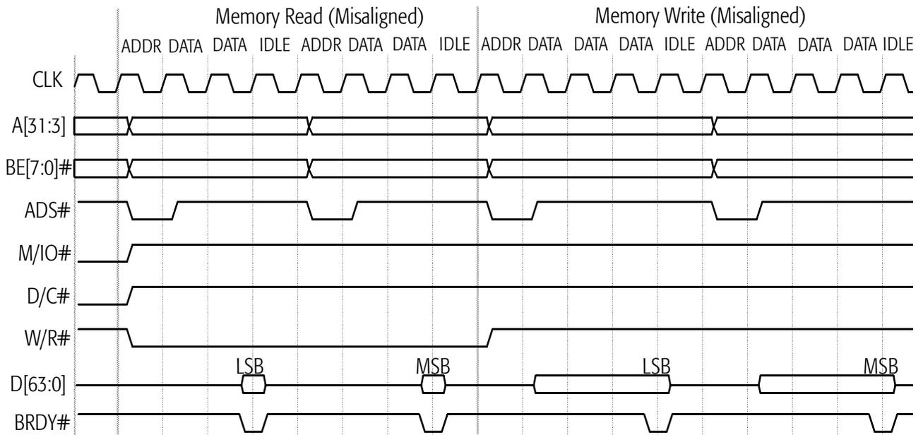
**Figure 46. Misaligned Single-Transfer Memory Read and Write**
