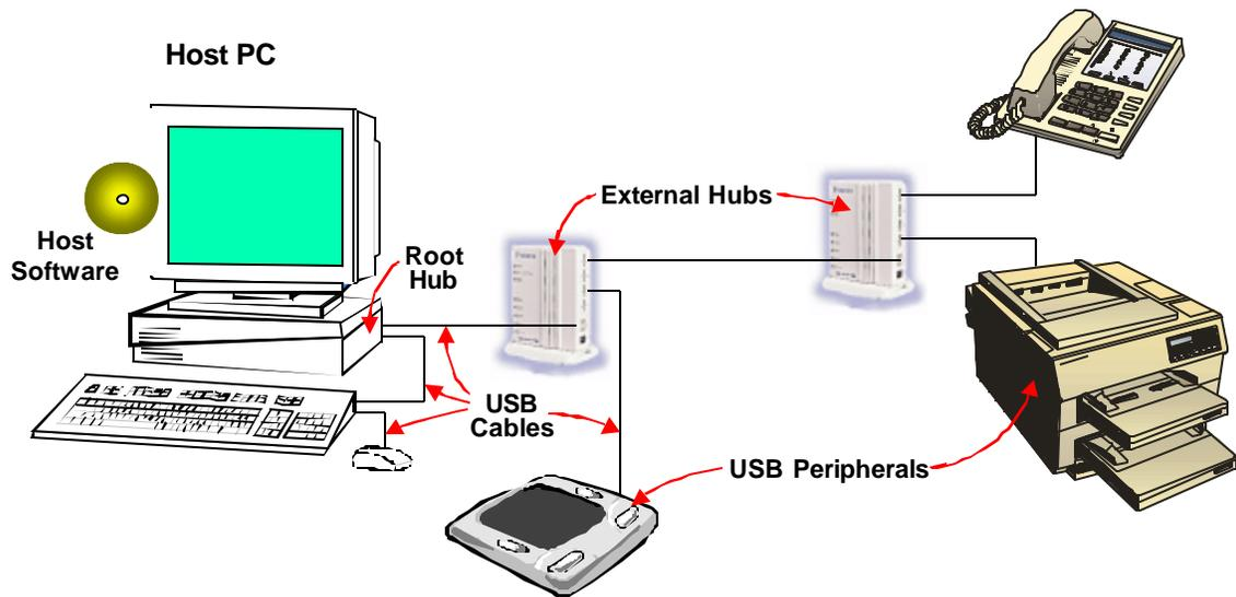
**Figure 1. USB 1.1 System Configuration**
