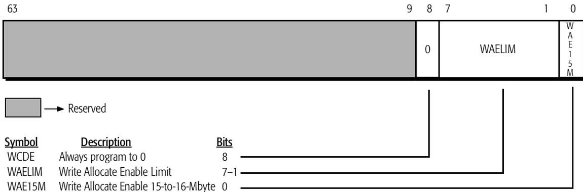
**Figure 32. Write Handling Control Register (WHCR)**
