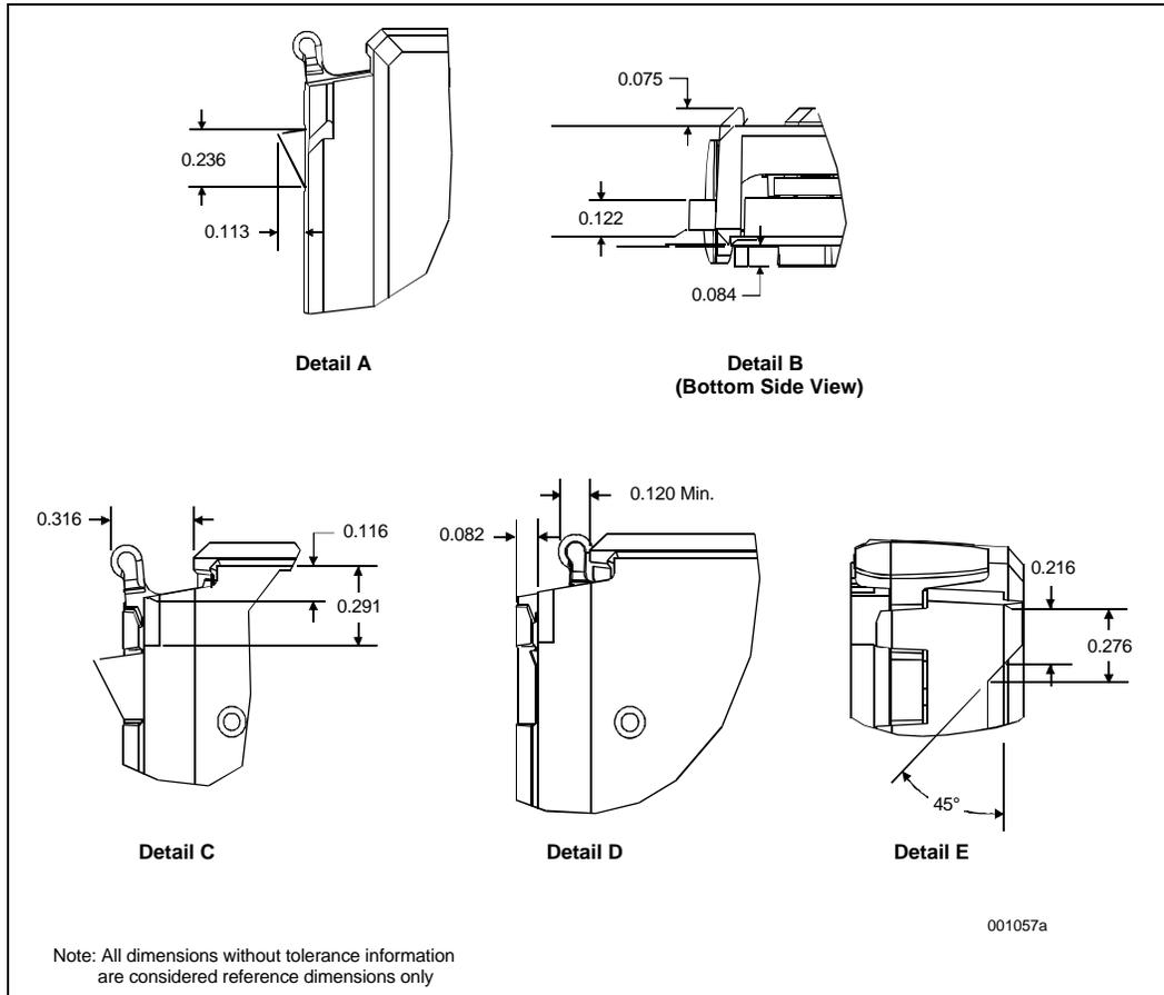
Figure 23. Pentium® II Processor (S.E.C.C. Package)—Extended Thermal Plate Attachment Detail Dimensions
