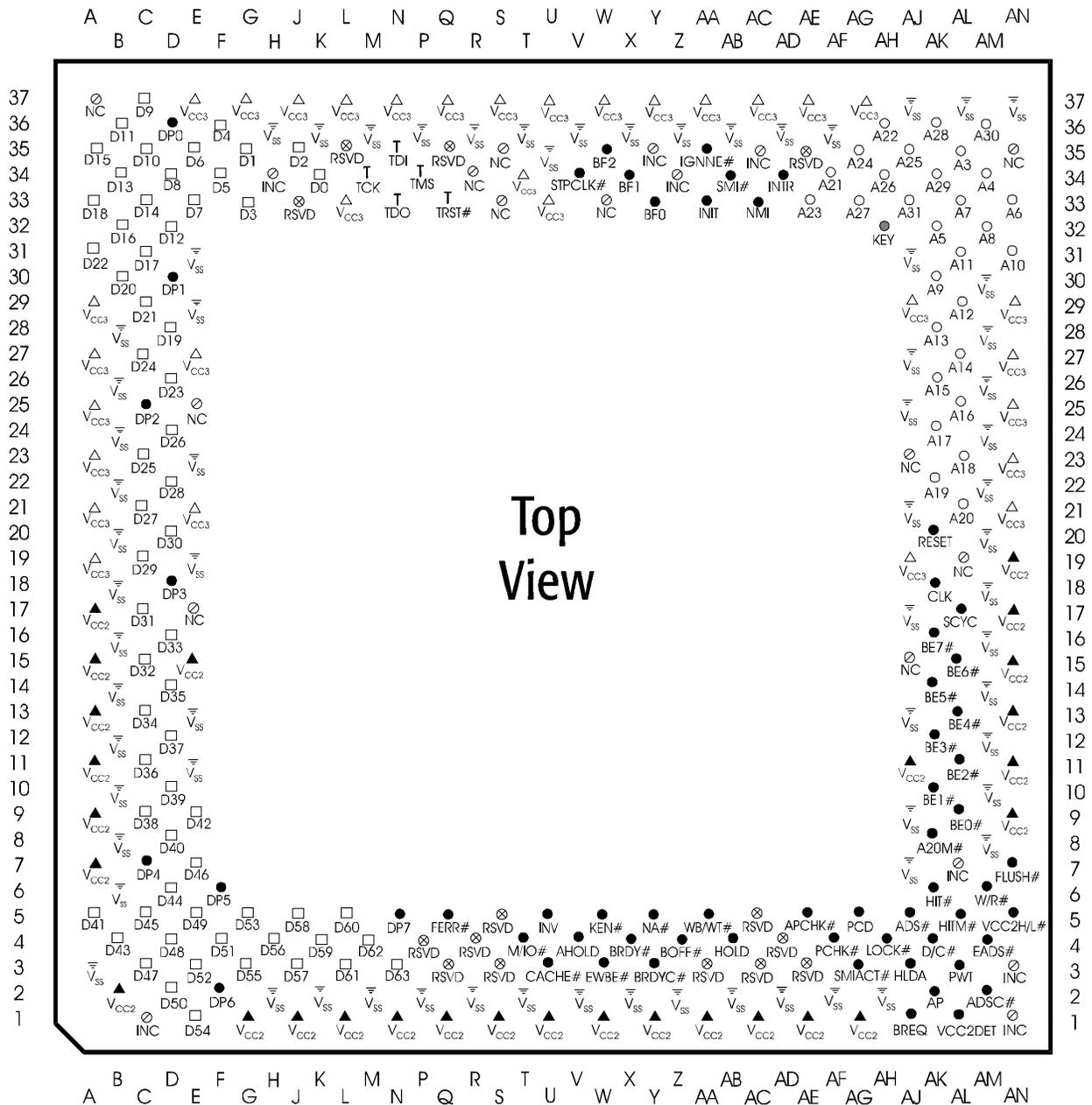
Figure 104. AMD-K6<sup>®</sup> Processor Model 7 Top-Side View
