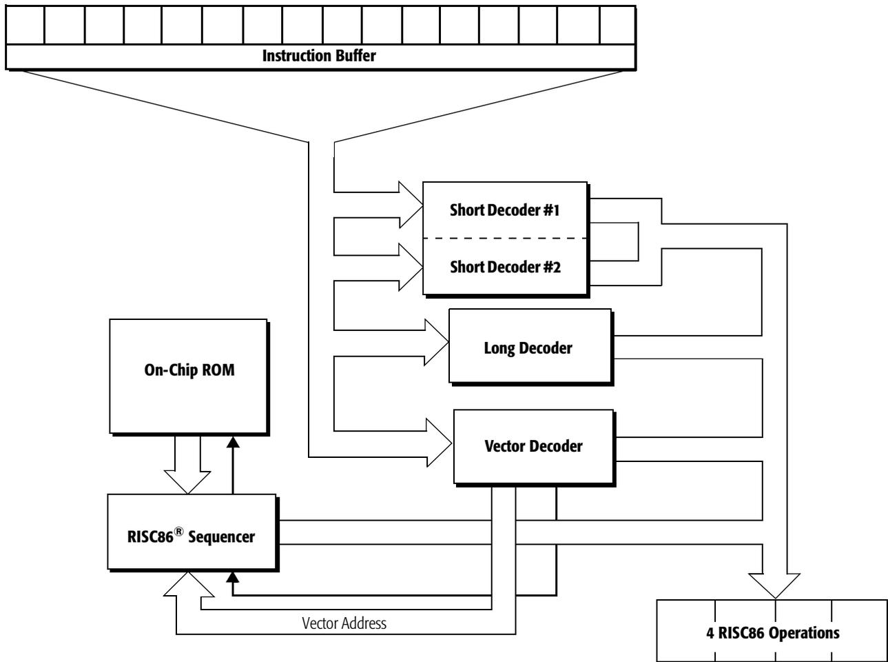
Figure 4. AMD-K6<sup>®</sup> Processor Decode Logic
