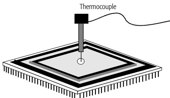
Figure 94. Measuring Case Temperature
