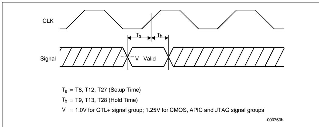
Figure 9. System Bus Reset and Configuration Timings
