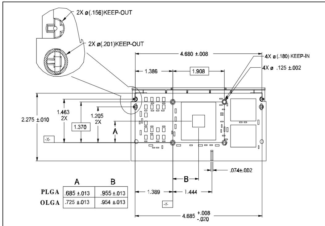
Figure 31. Pentium® II Processor Assembly (S.E.C.C.2 Package)—Cover View with Dimensions
