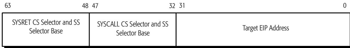
**Figure 103. SYSCALL/SYSRET Target Address Register (STAR)****Table 61. SYSCALL/SYSRET Target Address Register (STAR) Definition**
