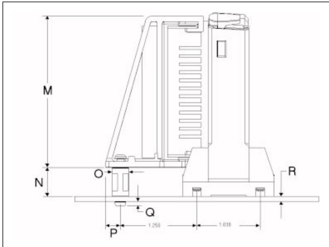
Figure 46. Top View Space Requirements for Boxed Processor Fan Heatsink Supports
