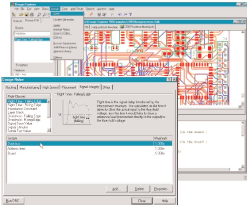
Protel 99 includes a comprehensive set of signal integrity design rules covering areas such as net impedance, overshoot, undershoot, flight time and signal slope. Signal integrity violations are then included as part of the standard board DRC report.
