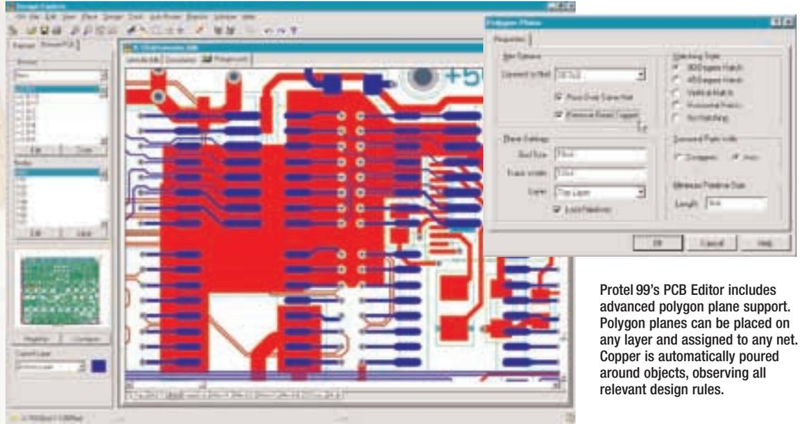
Protel 99's PCB Editor includes advanced polygon plane support. Polygon planes can be placed on any layer and assigned to any net. Copper is automatically poured around objects, observing all relevant design rules.
