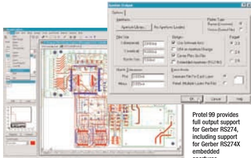
Protel 99 provides full output support for Gerber RS274, including support for Gerber RS274X embedded apertures.
