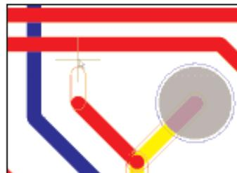
Protel 99's "avoid obstacle" manual routing mode automatically clips the track you are placing to avoid creating design rule violations. This makes it easy to "slam-and-jam" tracks together while maintaining defined clearances.
