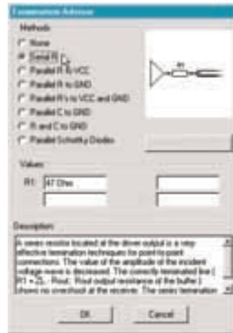
The integrated Termination Advisor allows you to experiment with different termination options for each connection, then run a virtual simulation using the selected termination. Find the optimal solution before modifying your board.
