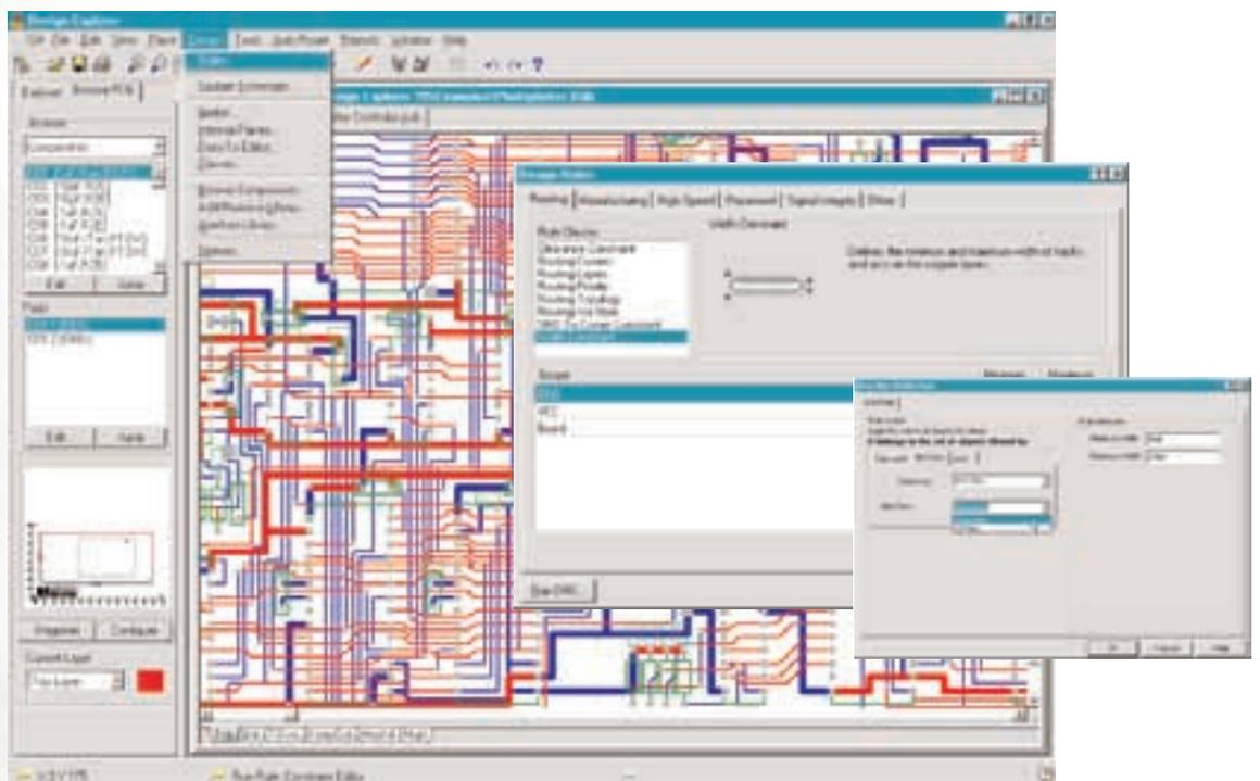
Protel 99's PCB Editor incorporates over 25 design rule classes covering areas such as routing, manufacturing, high-speed design, component placement, and signal integrity. Combined with the ability to create multiple rules, each with a different scope, Protel 99 gives you total control over the design process. The ability to create compound rule scopes allows you to precisely target the objects a rule applies to.
