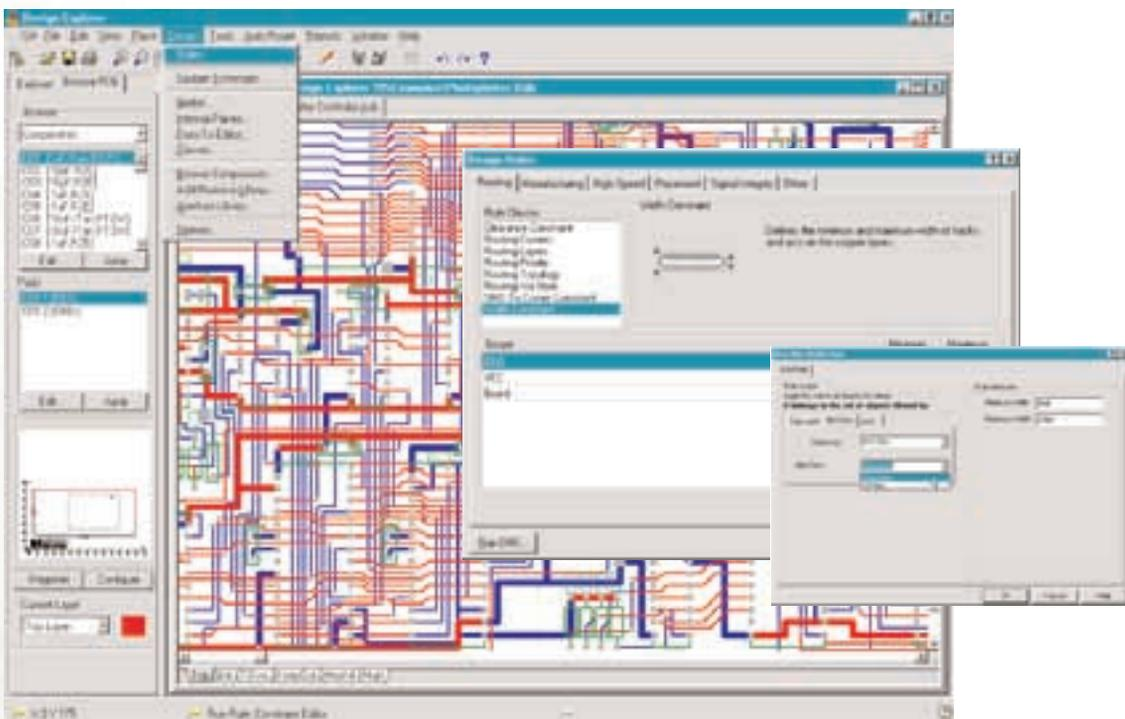
Protel 99's PCB Editor incorporates over 25 design rule classes covering areas such as routing, manufacturing, high-speed design, component placement, and signal integrity. Combined with the ability to create multiple rules, each with a different scope, Protel 99 gives you total control over the design process. The ability to create compound rule scopes allows you to precisely target the objects a rule applies to.
