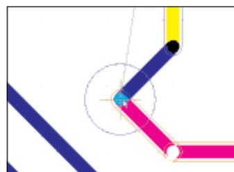
The PCB's special "electrical grid" feature snaps the cursor to valid electrical connection points, regardless of the current routing grid setting. This makes it easy to route to off-grid pads and tracks, enabling virtually gridless manual routing.
