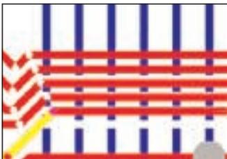
Effortlessly route through tight spaces using the "push-and-shove" manual routing mode. Existing tracks are pushed out of the way in accordance with all relevant design rules.
