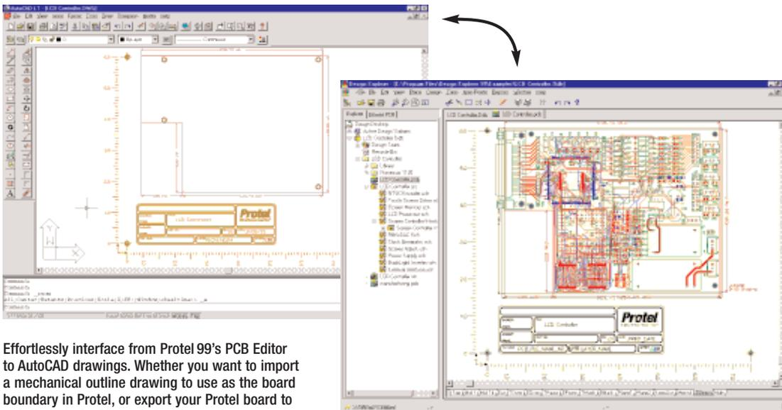
Effortlessly interface from Protel 99's PCB Editor to AutoCAD drawings. Whether you want to import a mechanical outline drawing to use as the board boundary in Protel, or export your Protel board to AutoCAD, Protel 99's AutoCAD translator makes it easy. The translator imports/exports both DXF and DWG files, as well as supporting user-defined layer mapping and PCB component - AutoCAD block transforms.
