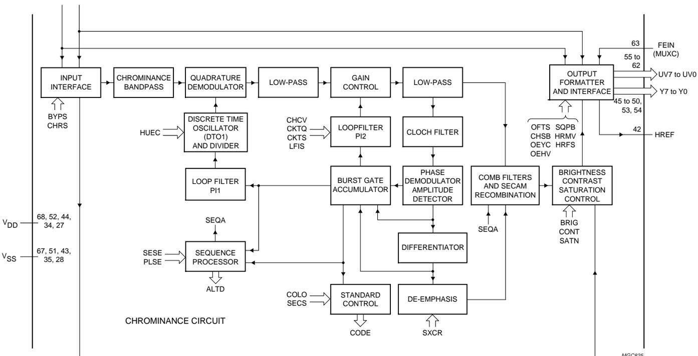
Fig.6 Multi-standard decoder part.
