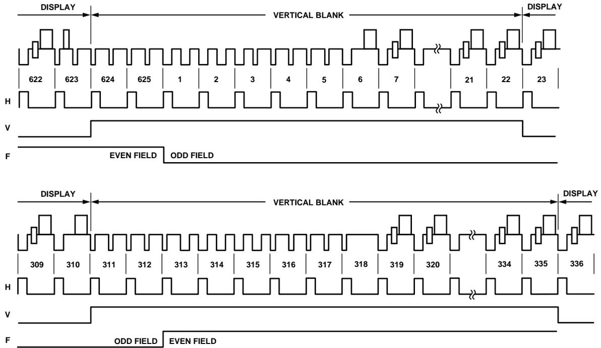
Figure 22. Timing Mode 0 (PAL Master Mode)
