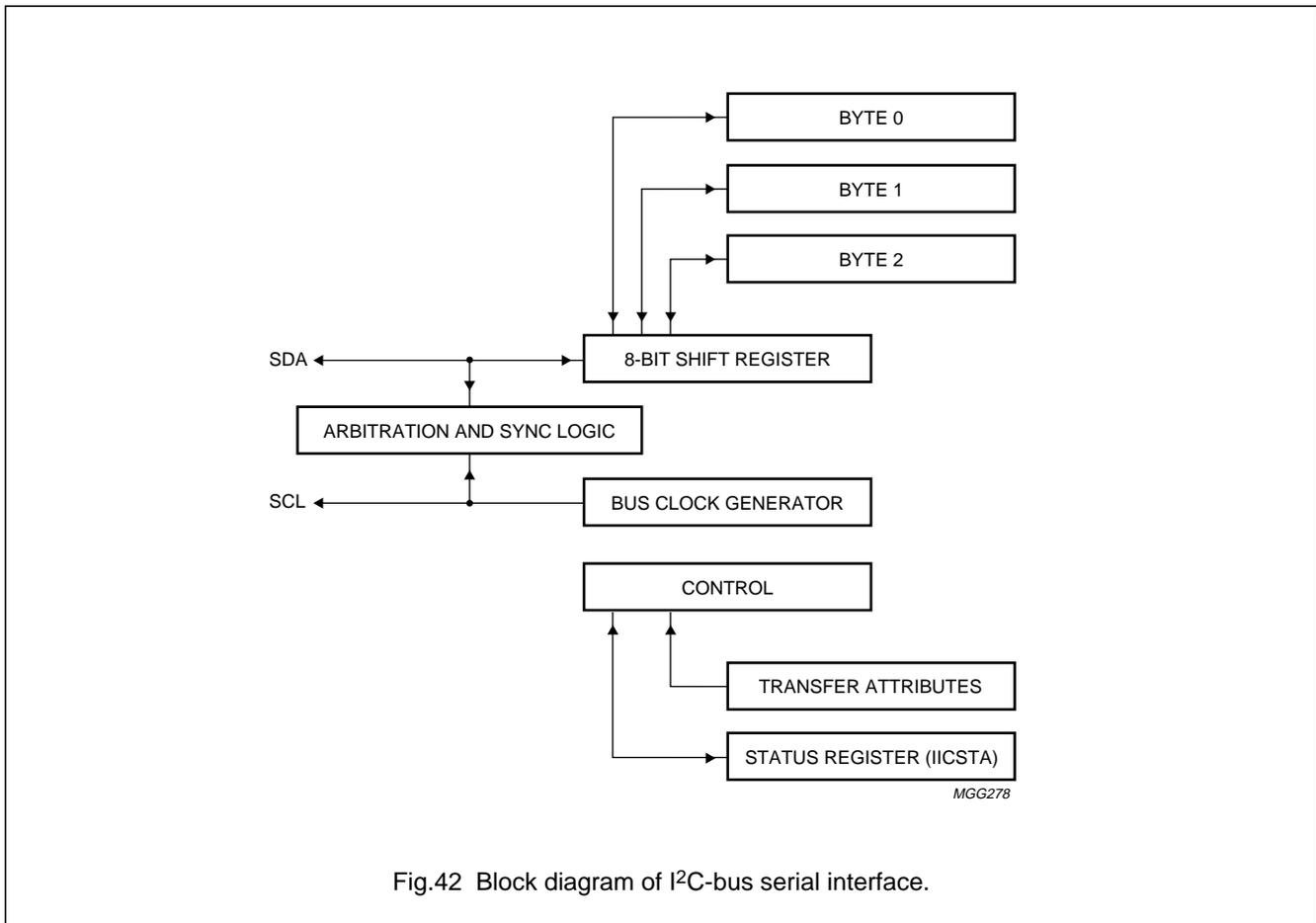
Fig.42 Block diagram of I<sup>2</sup>C-bus serial interface.
