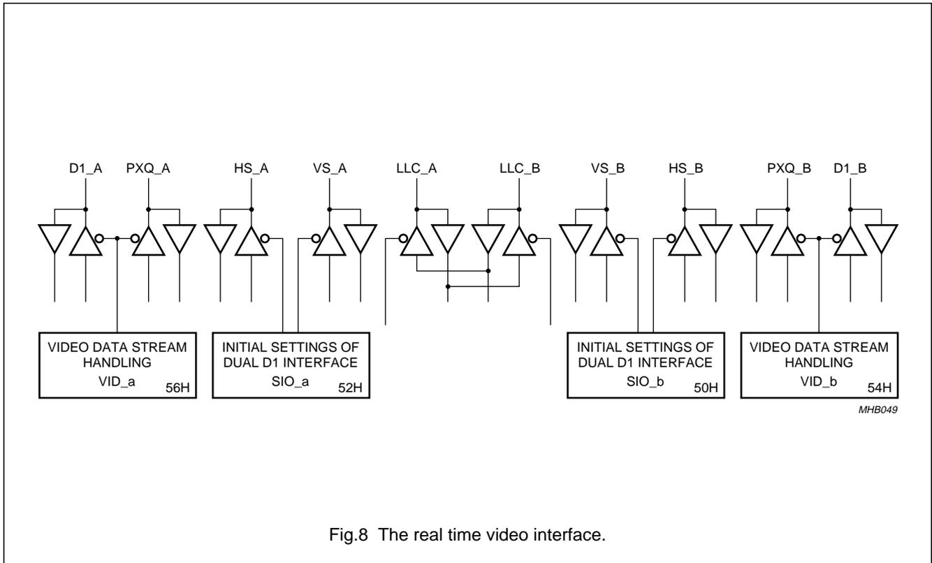
Fig.8 The real time video interface.
