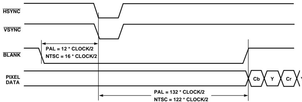
Figure 29. Timing Mode 2 Even-to-Odd Field Transition Master/Slave
