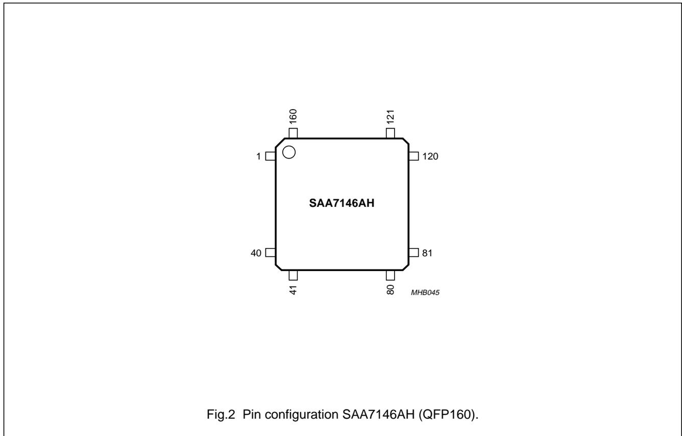
Fig.2 Pin configuration SAA7146AH (QFP160).
