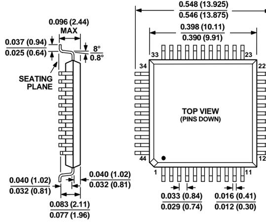
44-Lead Thin Plastic Quad Flatpack (TQFP)
