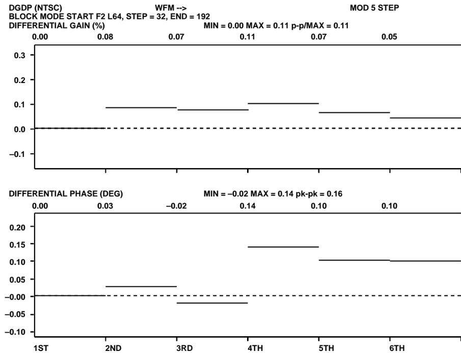
Figure 94. NTSC Differential Gain and Phase Measurement
