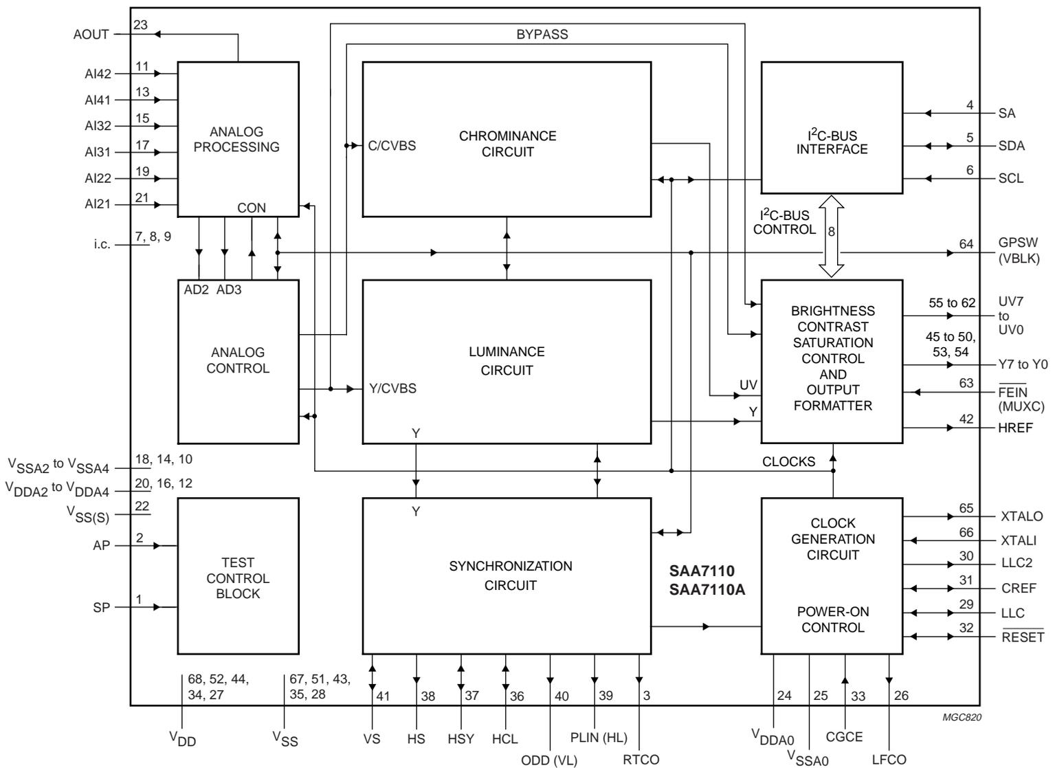
Fig.2 Block diagram.
