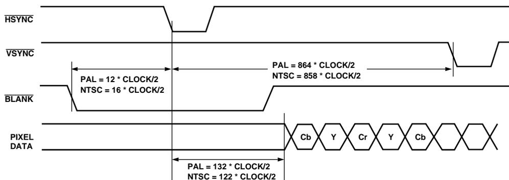
Figure 30. Timing Mode 2 Odd-to-Even Field Transition Master/Slave
