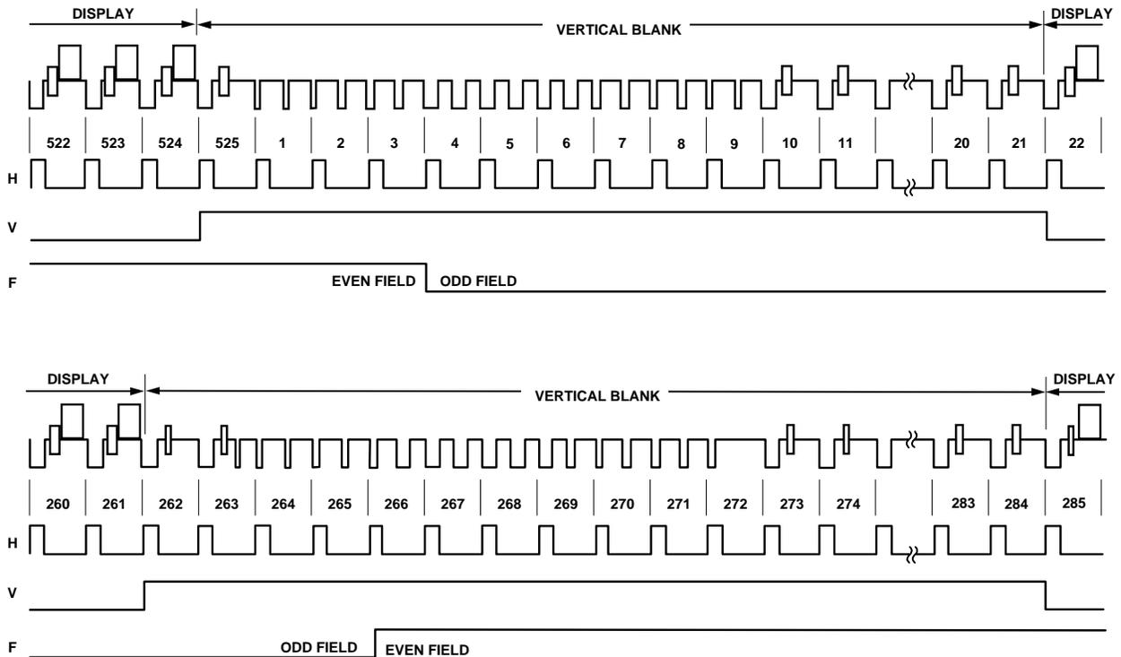
Figure 21. Timing Mode 0 (NTSC Master Mode)
