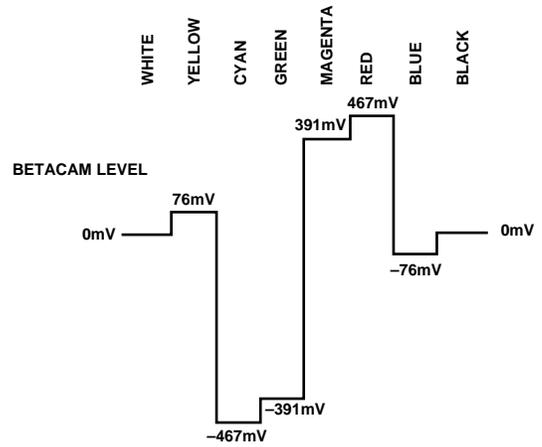
Figure 77. NTSC 100% Color Bars with Pedestal V Levels
