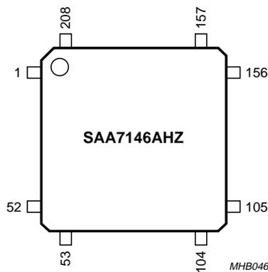
Fig.3 Pin configuration SAA7146AHZ (SQFP208).
