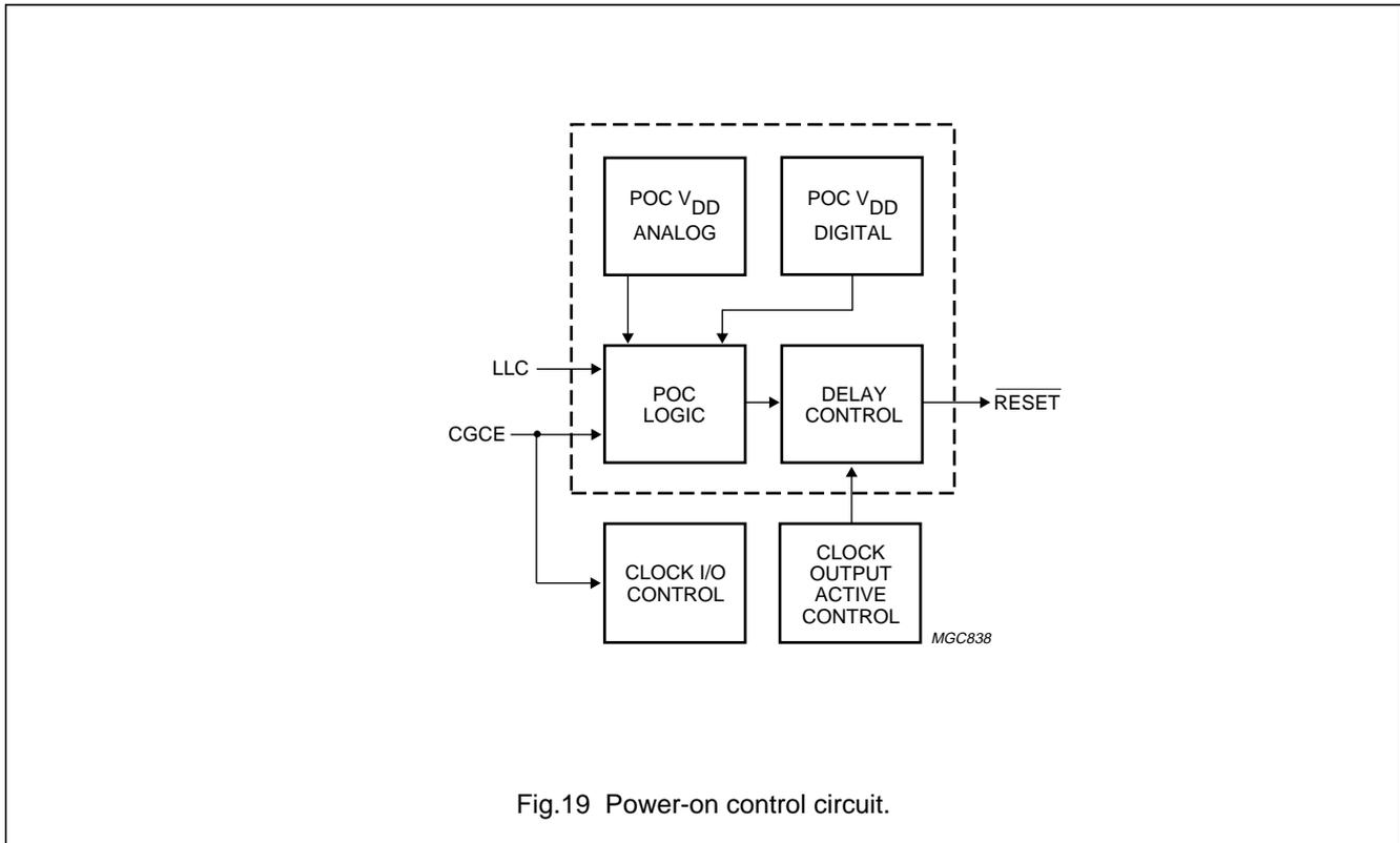
Fig.19 Power-on control circuit.
