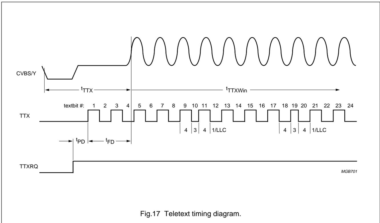
Fig.17 Teletext timing diagram.
