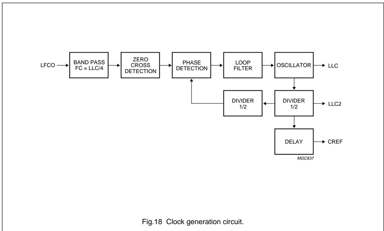
Fig.18 Clock generation circuit.
