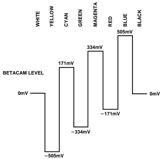
Figure 73. NTSC 100% Color Bars, No Pedestal U Levels
