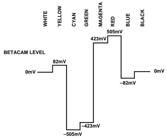
Figure 76. NTSC 100% Color Bars, No Pedestal V Levels
