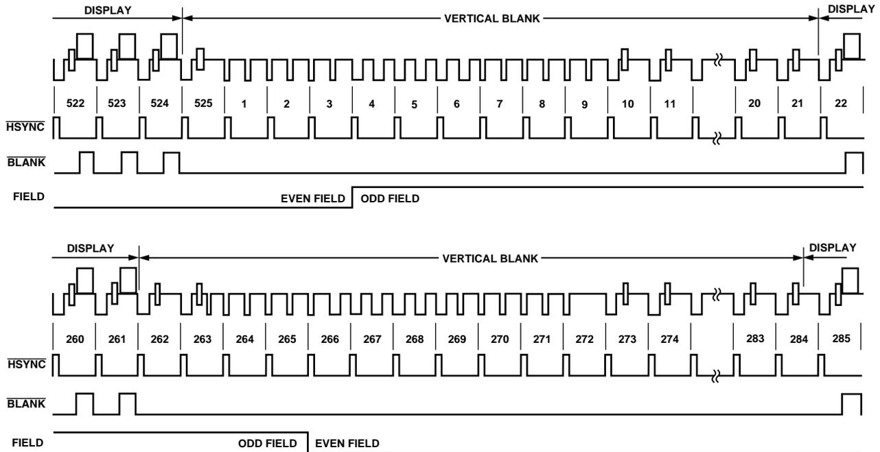
Figure 31. Timing Mode 3 (NTSC)
