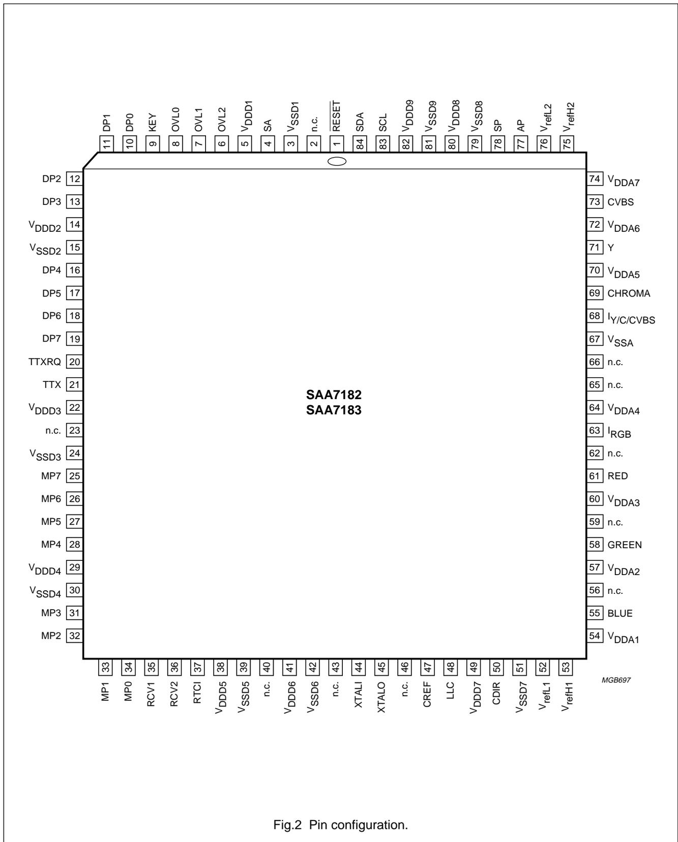
Fig.2 Pin configuration.
