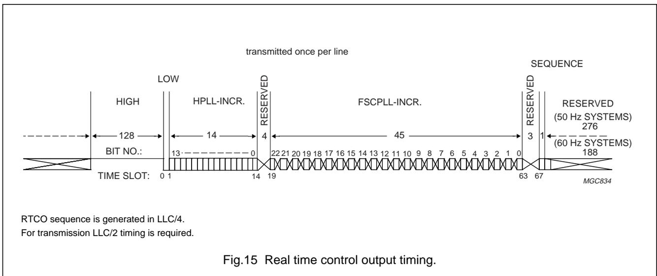
Fig.15 Real time control output timing.
