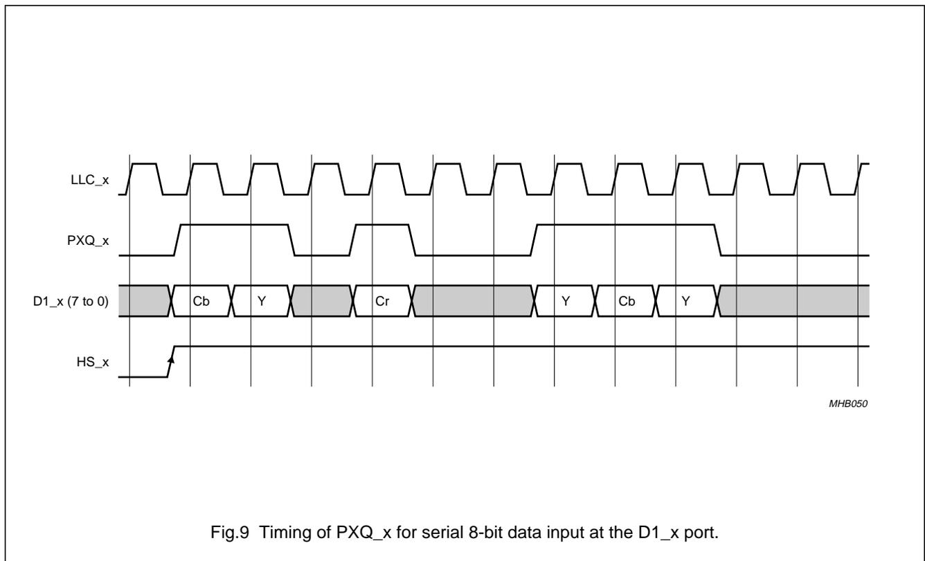
Fig.9 Timing of PXQ\_x for serial 8-bit data input at the D1\_x port.
