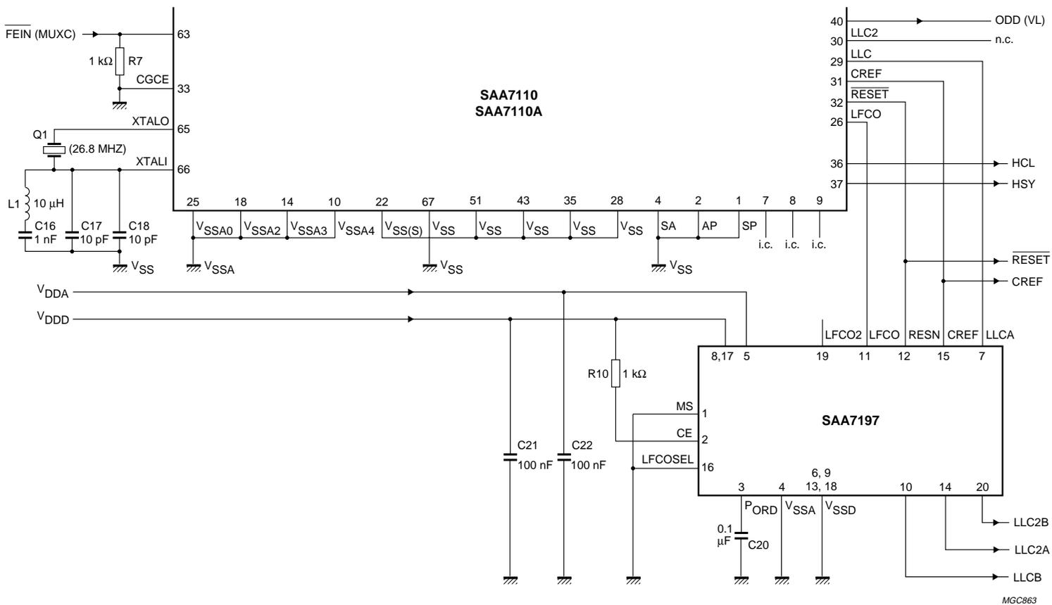
The OCF1 supports for special applications the use of an external CGC (SAA7197). For normal operation the built-in CGC fulfils all requirements.
