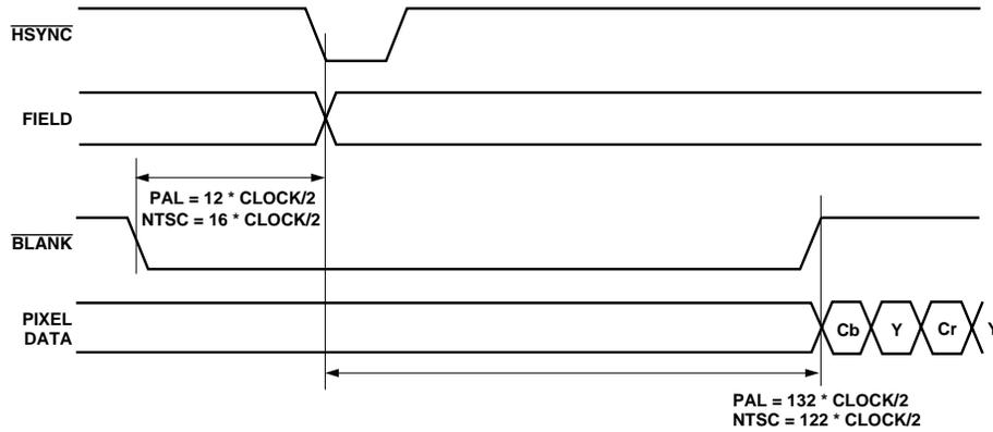
Figure 26. Timing Mode 1 Odd/Even Field Transitions Master/Slave
