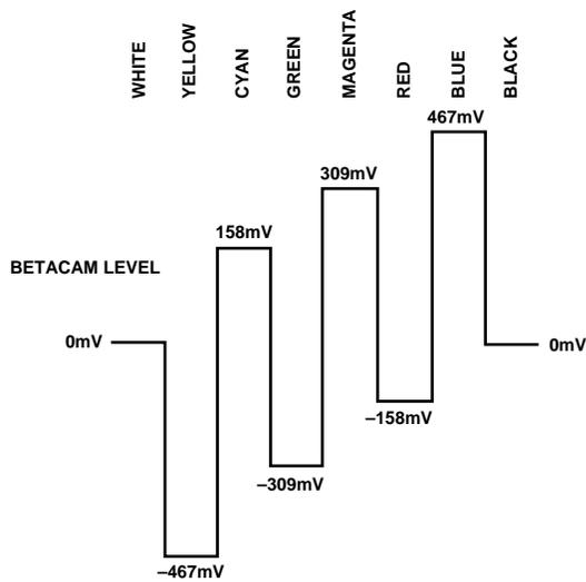
Figure 74. NTSC 100% Color Bars with Pedestal U Levels
