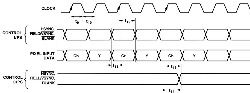
Figure 2. Pixel and Control Data Timing Diagram
