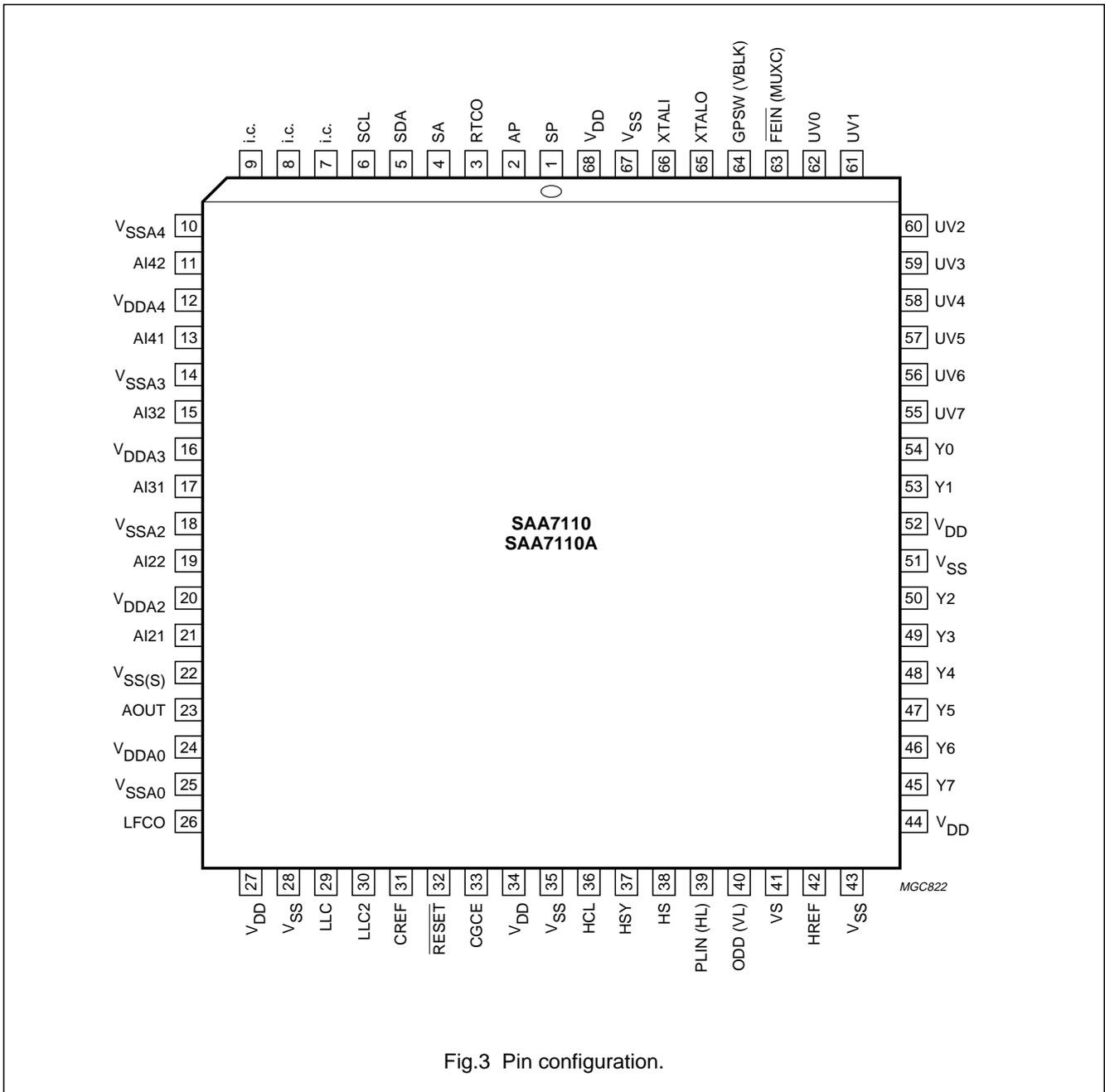
Fig.3 Pin configuration.
