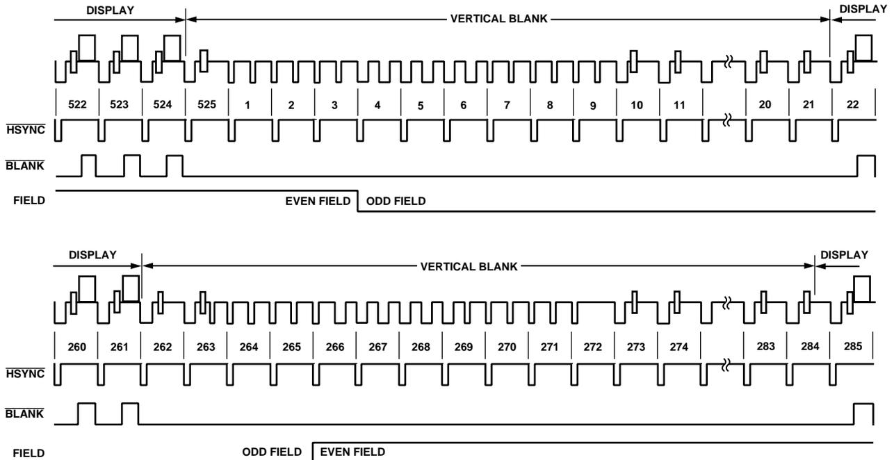
Figure 24. Timing Mode 1 (NTSC)
