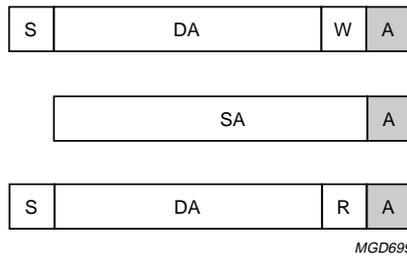
Fig.44 Address slave and write to IICTFR.
