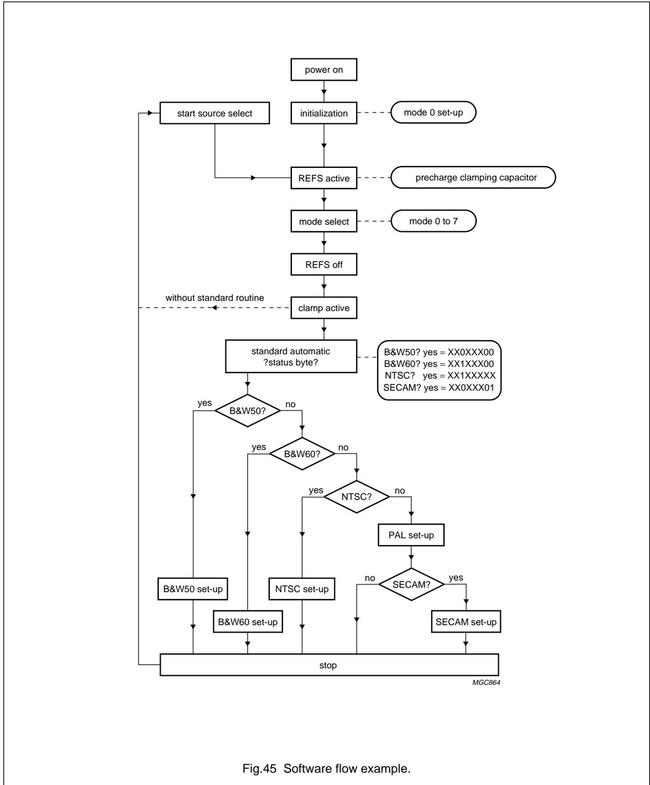
Fig.45 Software flow example.
