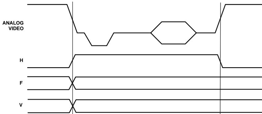
Figure 23. Timing Mode 0 Data Transitions (Master Mode)
