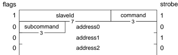
Figure 25—Write request packet format
