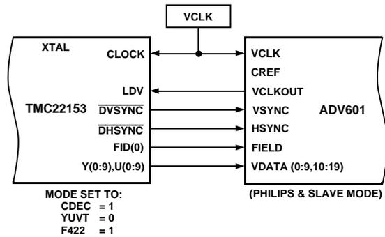
Figure 21. ADV601 and TMC22153 Example Philips-Like Mode Interface
