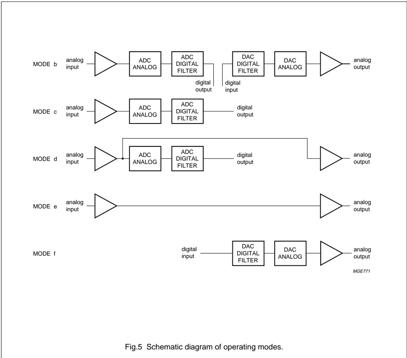
Fig.5 Schematic diagram of operating modes.
