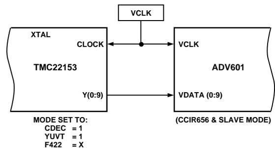
Figure 22. ADV601 and TMC22153 Example CCIR-656 Mode Interface
