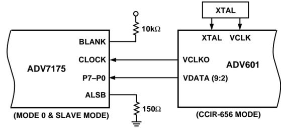
Figure 20. ADV601 and ADV7175 Example Interfacing Block Diagram
