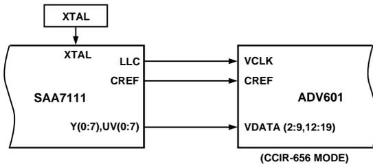
Figure 19. ADV601 and SAA7111 Example Interfacing Block Diagram
