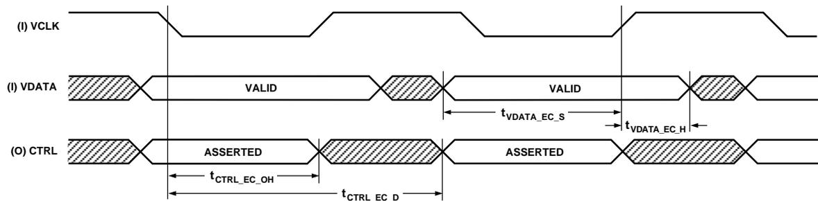
Figure 26. CCIR-656 Video—Encode Pixel (YCrCb) Transfer Timing
