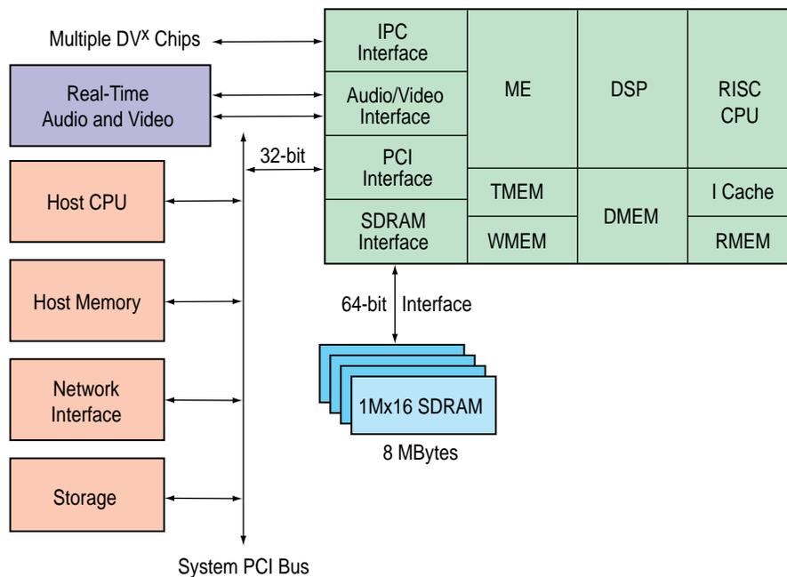
DV<sup>x</sup> Platform Architecture Block Diagram
