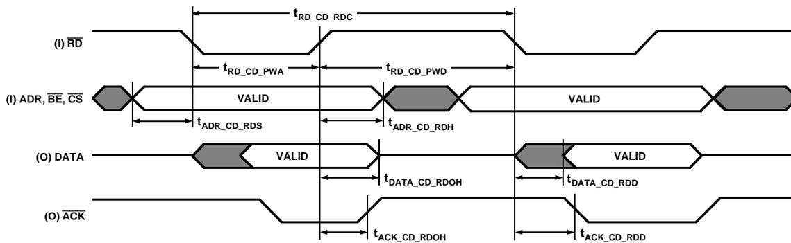
Figure 39. Host (Compressed Data) Read Transfer Timing
