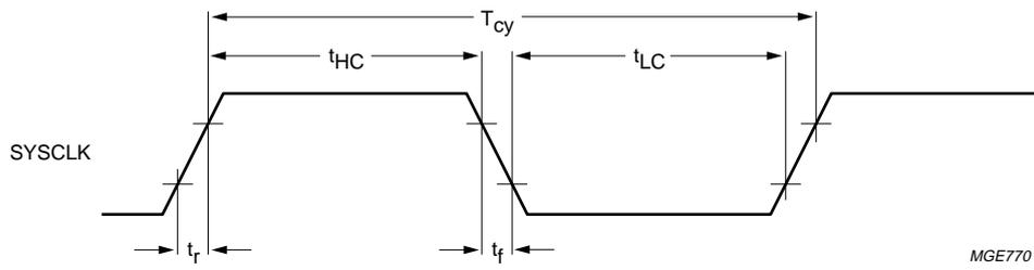
Fig.7 Serial timing of SYSCLK related signals.
