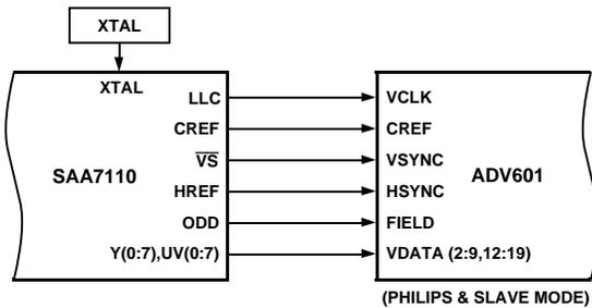
Figure 18. ADV601 and SAA7110 Example Interfacing Block Diagram
