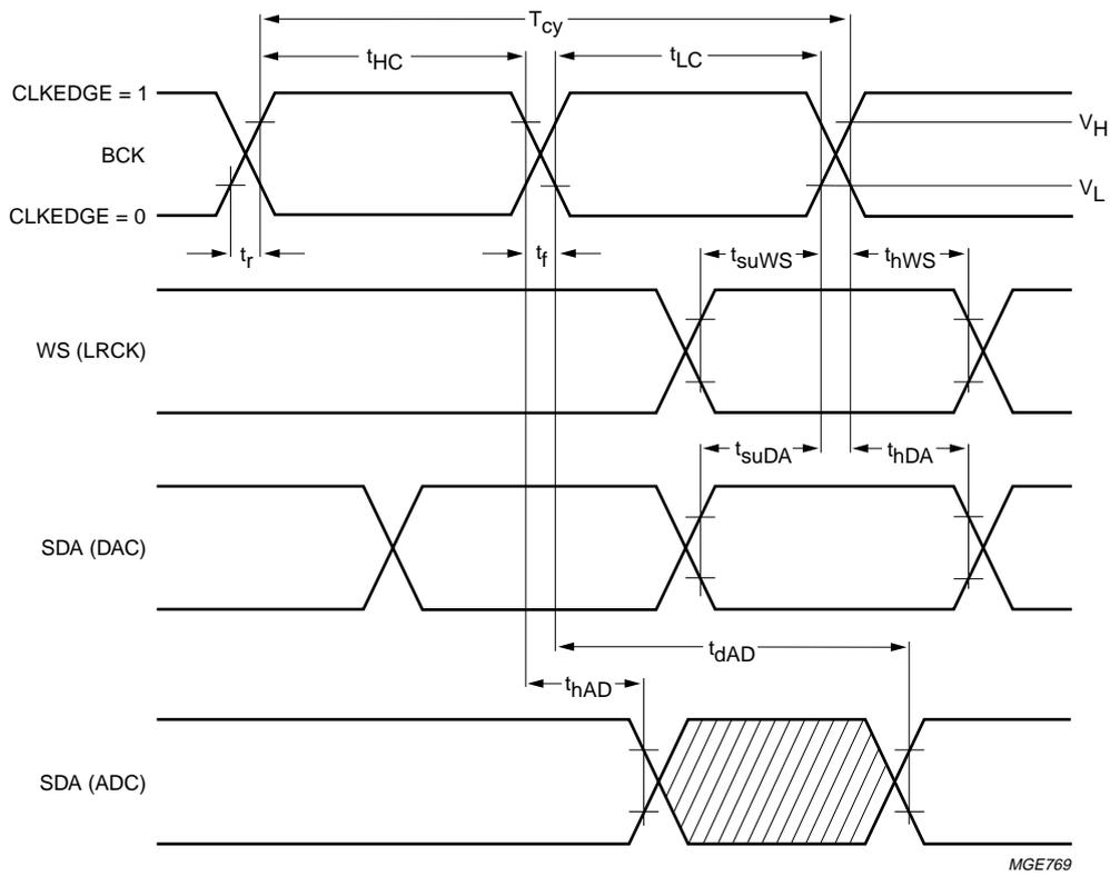
Fig.6 Serial timing of BCK related signals.
