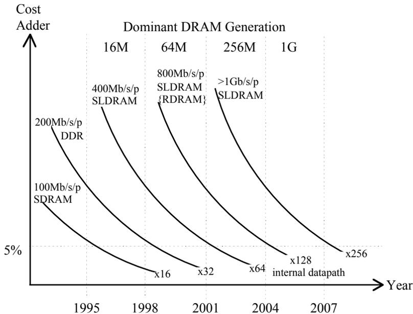
Figure 2. DRAM Bandwidth Cost Penalty for 16 bit I/O
