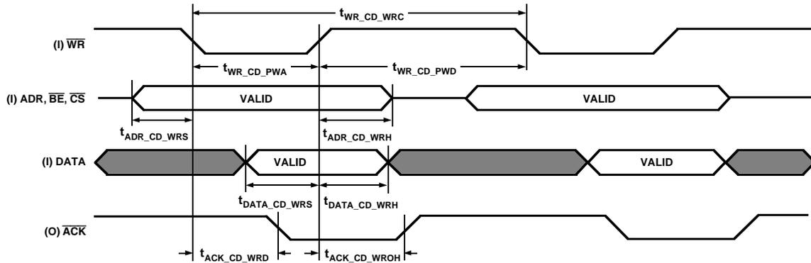
*Figure 40. Host (Compressed Data) Write Transfer Timing*
