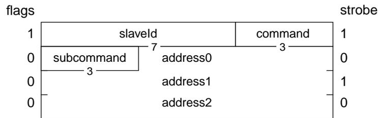
**Figure 21—Command/address packet components**
