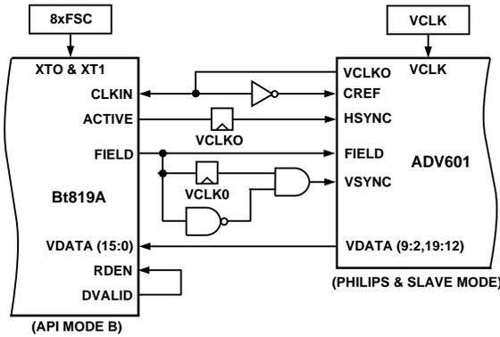
Figure 17. ADV601 and Bt819A Example Interfacing Block Diagram
