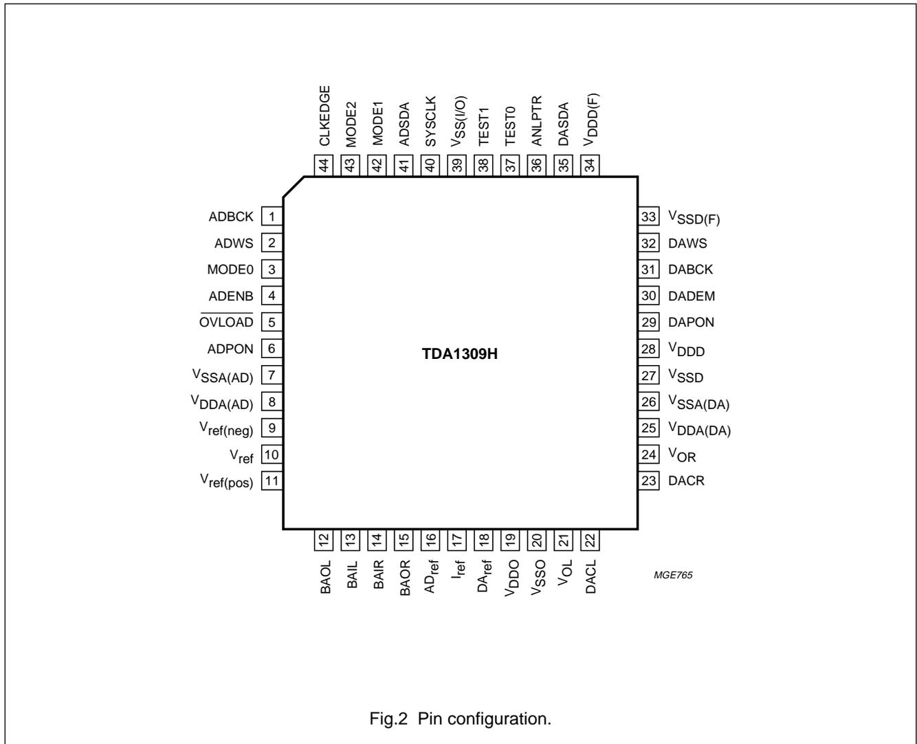
Fig.2 Pin configuration.
