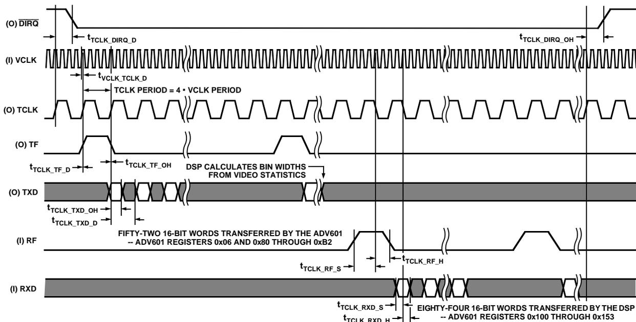
Figure 41. DSP Read and Write Transfer Timing
