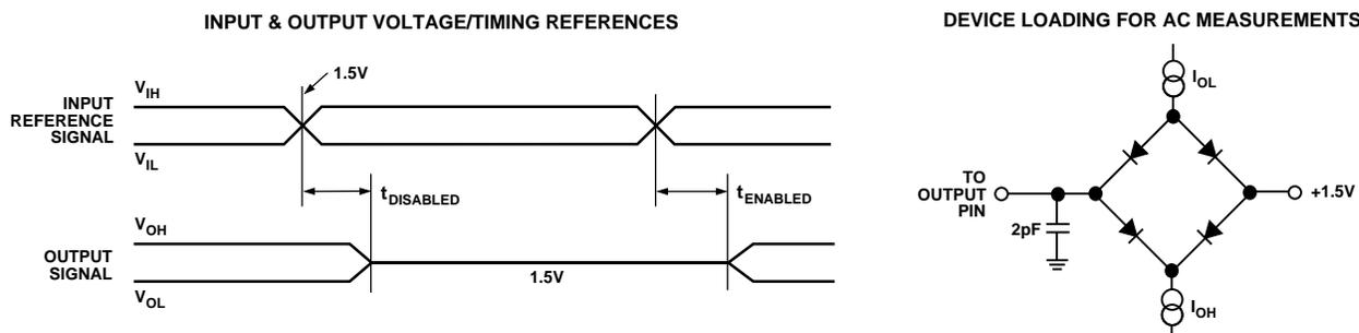
Figure 23. Test Condition Voltage Reference and Device Loading
