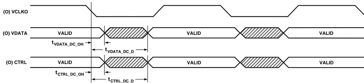
Figure 25. CCIR-656 Video—Decode Pixel (YCrCb) Transfer Timing
