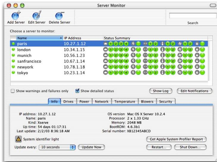
Server Monitor is an advanced software tool that provides feedback on hardware status. Red, yellow, and green lights indicate the health of each server, which is identified by name and IP address. Next to each server name is at-a-glance summary information for each subsystem. A click on any of the status icons opens the corresponding tab for instant retrieval of status and performance details.
