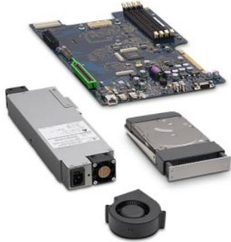
AppleCare Service Parts Kits for Xserve include a power supply, blower, logic board, and Apple Drive Module.
