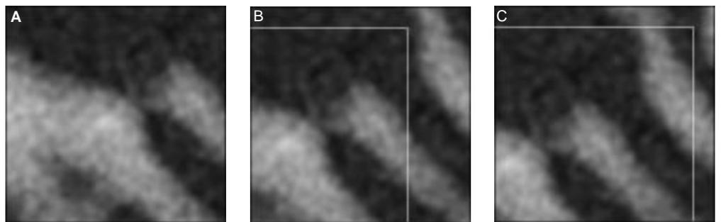
Corresponding series of images fed to the DSP for processing. The white lines mark the overlap with the previous image.
