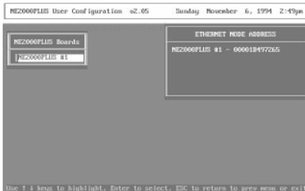
5. There's only one NE2000 in the machine, so it is the only one listed. Press *Enter* to get the configuration screen.
