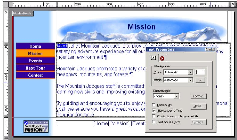
Notice the text box has a wide border and does not show any object handles. This is because the default option for imported text is **Size Layout to Text**. When this option is selected, the text assumes the size of the Layout, and you cannot resize the text box.
