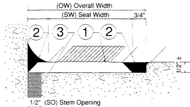
1. ISO-FLEX WS Series Polyurethane Seal
