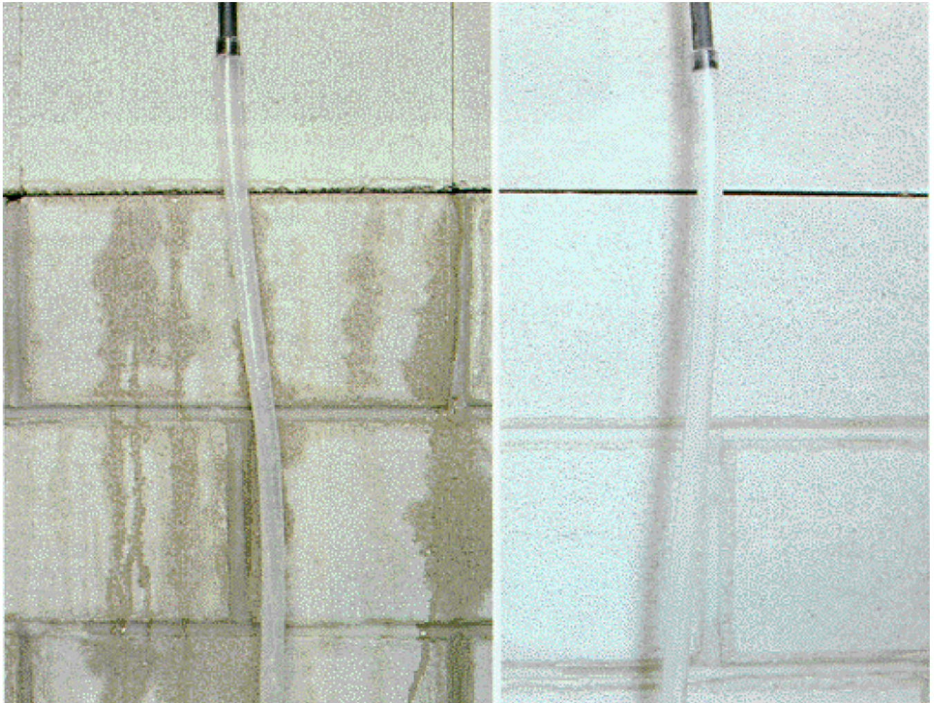
Demonstration wall interior surfaces after a simulated 24 inch (60 cm) rainfall. Ordinary block wall (left) CONTROL-BLOK wall (right).
