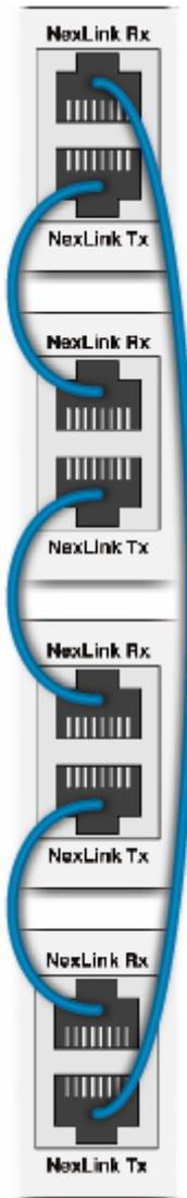
Up to four NEXIA devices may be linked together to share digital audio signals. Tx on one NEXIA device is connected to RX on the next device. NexLink utilizes standard CAT5 cabling, with a maximum recommended length of 5 meters per cable.
