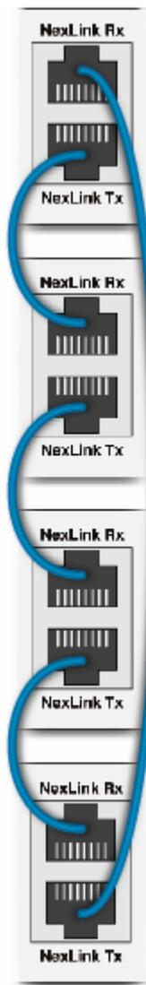
Up to four NEXIA devices may be linked together to share digital audio signals. Tx on one NEXIA device is connected to RX on the next device. NexLink utilizes standard CAT5 cabling, with a maximum recommended length of 5 meters per cable.
