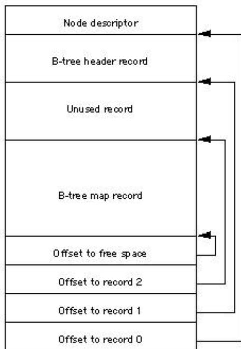
Figure 3 Header node structure
