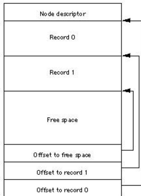
Figure 2. The structure of a node.
