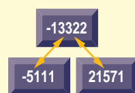
FIGURE 8 The Heap is On. Remember all the trouble you had with binary trees when you were still in school? The Heap sort is built on the principle of balancing a binary tree. Phase I is to build the heap. Phase II is to sort the tree. The Heap sort is not recursive, but it's still fast.
