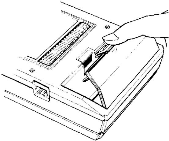
2. Insert four "C"-size carbon zinc or alkaline batteries (not included) into the battery compartment. Be sure that the positive (+) or cap ends of each battery are installed as shown inside the battery compartment.
