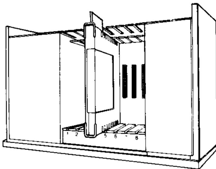
6. Replace the top on the Peripheral Expansion System by sliding the front edge under the extension on the front of the unit and firmly pressing down on the back edge of the top. Do not run the system without the top in place because the top ensures proper ventilation. *Note:* If the top does not fit properly, remove the card and realign it in the slot, remembering to press down firmly until the connection is made.
