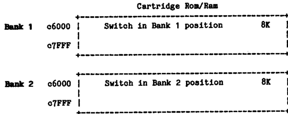
**NOTE:** The Cartridge Rom/Ram space in the Gram Kracker resides in CPU Memory and it is actually two different 8K chips that reside in the same address space at different times.
