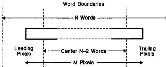
Figure 13-10. Pixel Block Alignment in X
