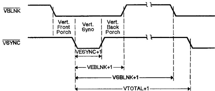
Figure 9-5. Vertical Timing for Noninterlaced Display
