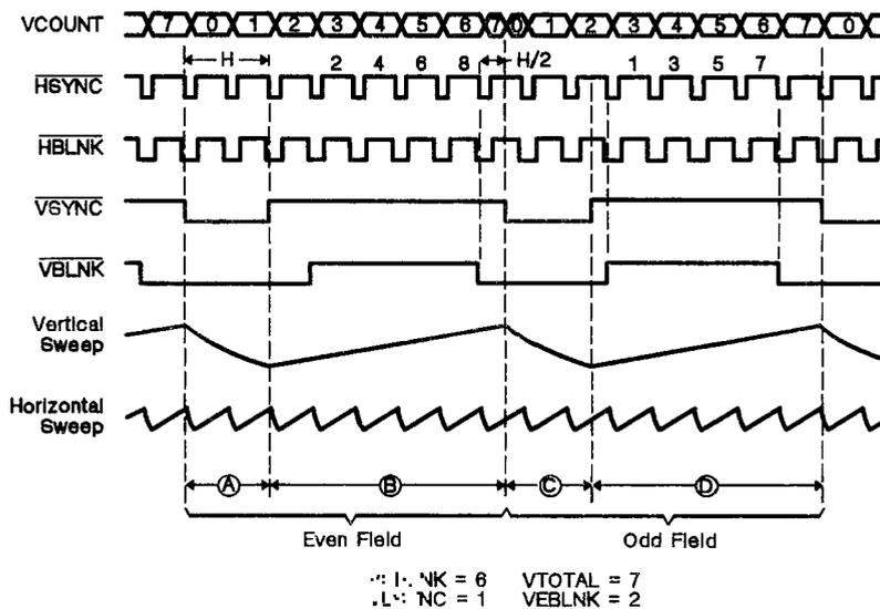
Figure 9-10. Interlaced Video Timing Waveform Example
