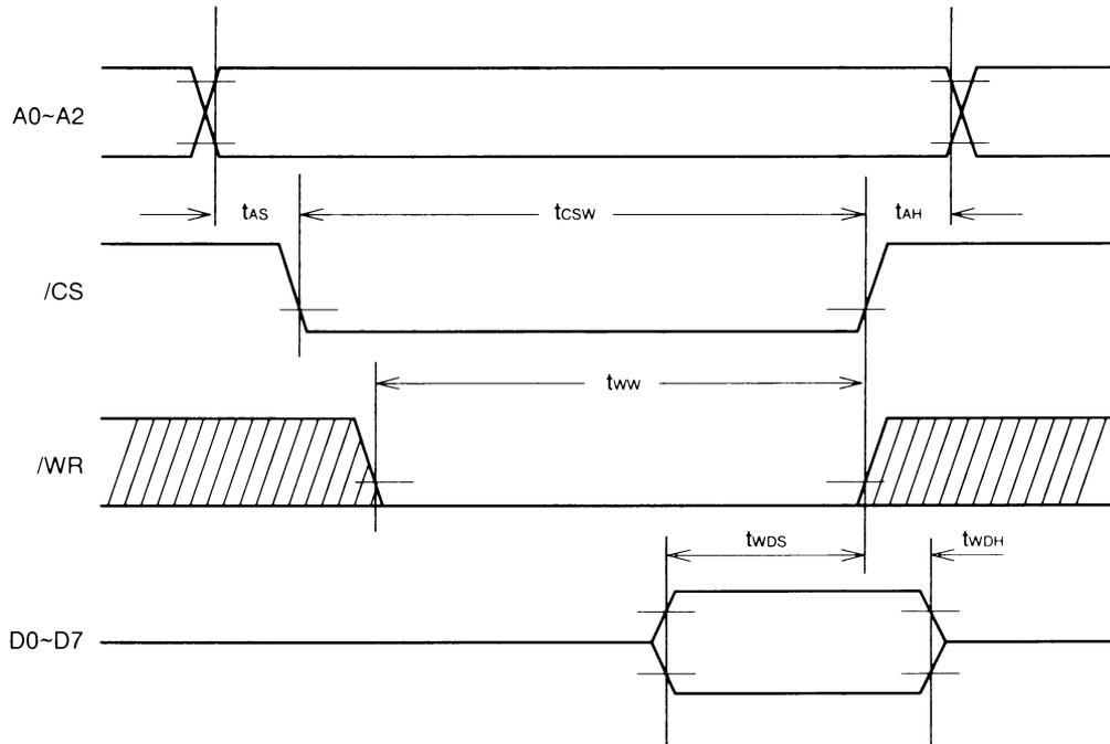
Note: tCSW, tWW, and tWDH are based on either /CS or /WR being driven to High level.
