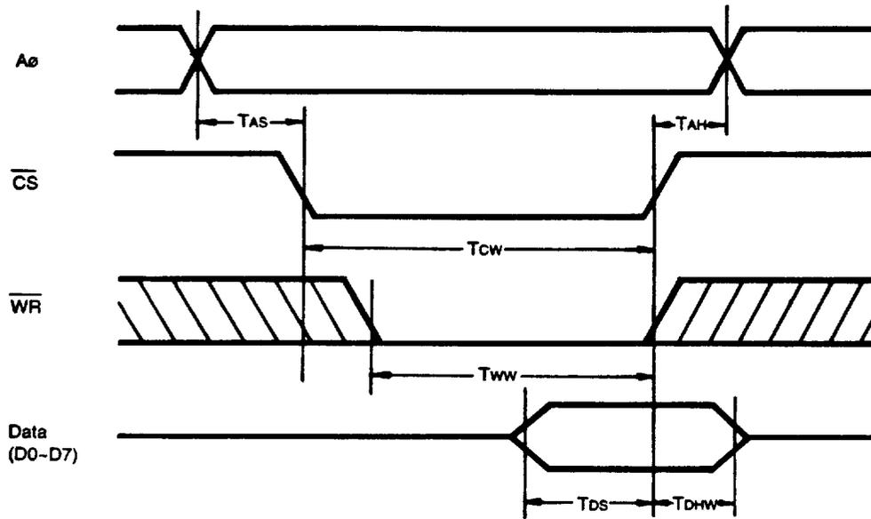
Fig 2-1 WRITE TIMING
