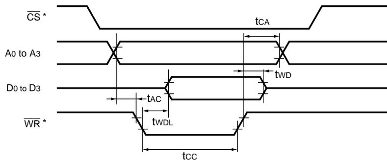
\*) The RP/RF5C01A accept  $\overline{WR}$  signals only when  $\overline{CS}$ ="L" and CS="H". Although  $\overline{CS}$  timing is not specified for the RP/RF5C01A, substitute  $\overline{WR}$  signals shown above with  $\overline{CS}$  ·  $\overline{WR}$  signals to be applicable to the RP/RF5C01A configuration.
