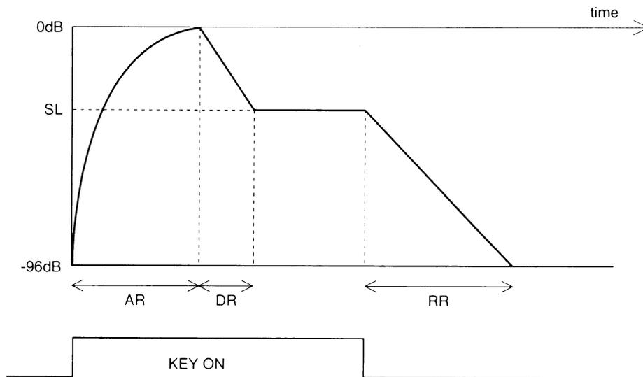
This envelop has a dynamic range of 96dB (resolution: 0.1875dB) and is expressed by damping amount.
