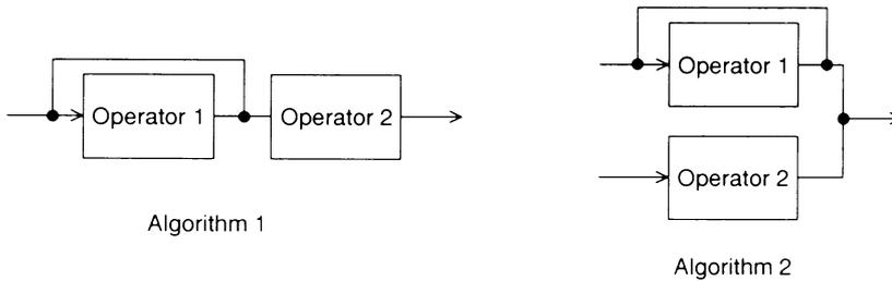
Registers C0 to C8H are set for each channel. Therefore, select algorithm 1 and 2 at each channel.
