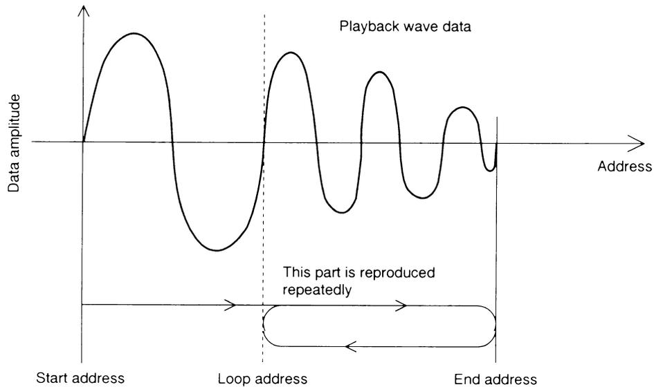
Note: A loop address and end address must be specified for all the sounds.
