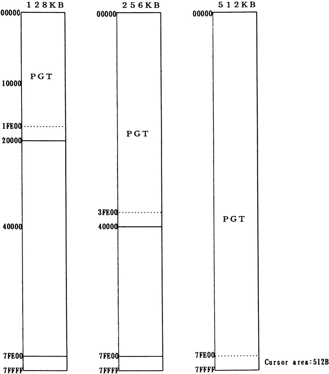
VRAM (256KB) to image space correspondence when the dot Number in the X direction of the image space is 512 at 8BIT/DOT in B1 mode.
