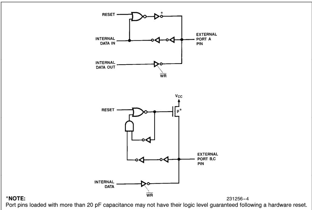
**\*NOTE:** Port pins loaded with more than 20 pF capacitance may not have their logic level guaranteed following a hardware reset.
