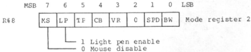
In addition, if you want to enable an interrupt when the light pen has detected light, set bit 5 of register R#0 to 1. This interrupt is reset if status register S#1 is read.
