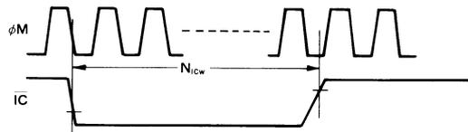
Fig. A-2 Reset Timing
