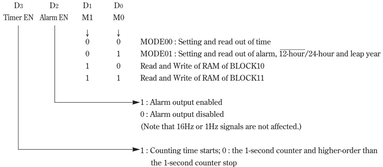
\*) When the Timer EN is set to 0, the 1-second counter and higher-order counters than the 1-second counter stop . If any carrying occurs in the lower-order counters than the 1 second counter while the Timer EN is 0, carrying will be held and avoided when the Timer EN changes from 0 to 1. Thus, no apparent delay is produced when the duration of the Timer EN = 0 is less than one second.
