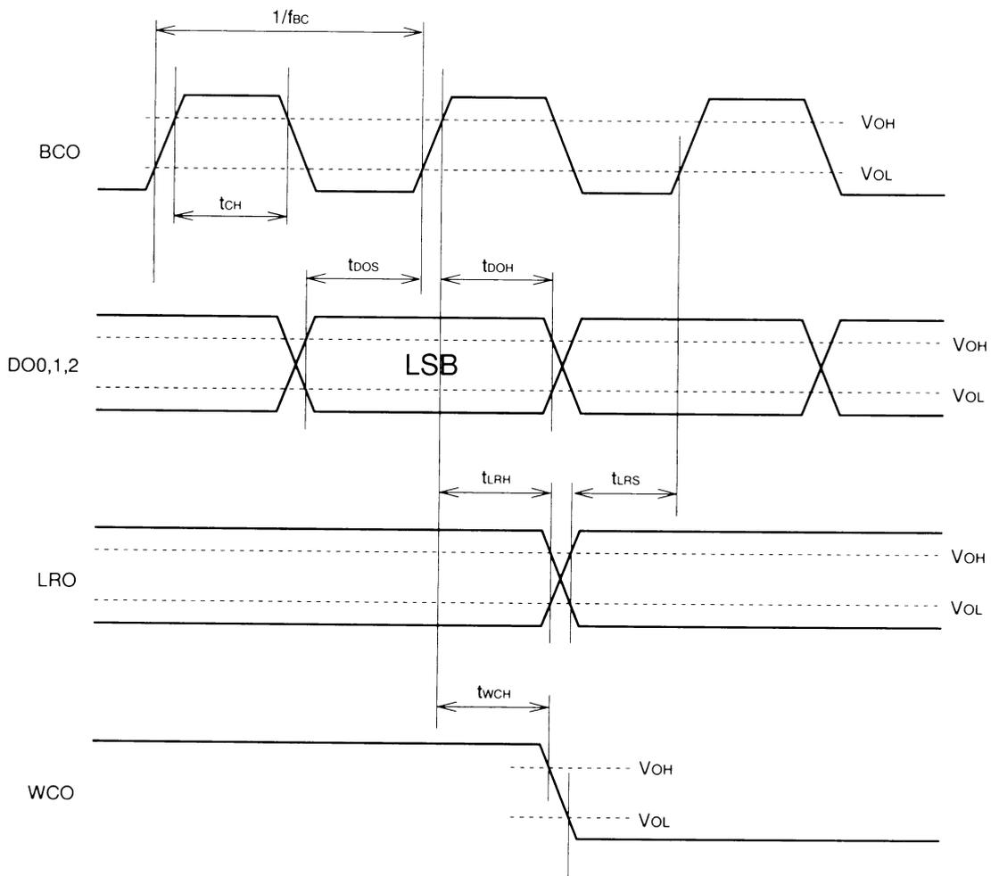
■ AC characteristics 3 Memory interface (conditions : Ta = 0~70°C, V<sub>DD</sub> = 5.0±0.25V)
