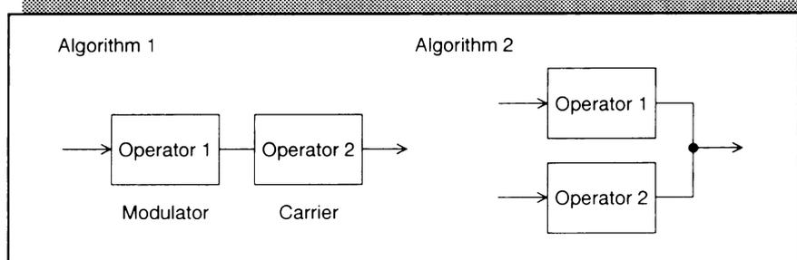
Algorithm 2 is the same regardless of the operator 1 and 2 slots. However, for algorithm 1, since the wave table depends on which slot is the carrier and which slot is the modulator, care must be given to the slot No.
