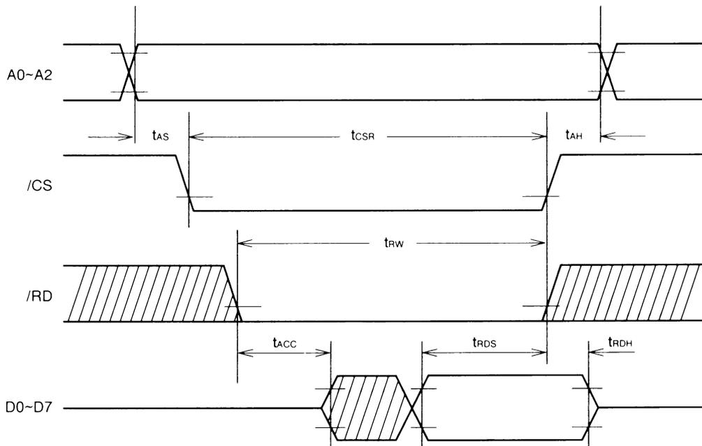
Note: tACC is based on whichever of /CS or /RD goes to the Low level last. tCSR, tRW, and tRDH are based on either /CS or /RD being driven to High level.
