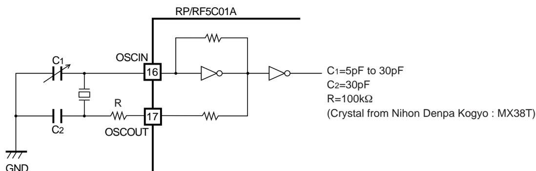
\*) Values of C<sub>1</sub>, C<sub>2</sub> and R are not absolute conditions but are indicated for reference only. Regard those C<sub>1</sub>, C<sub>2</sub> and R values shown above as our optimum values in our experiments which employed MX38T.
