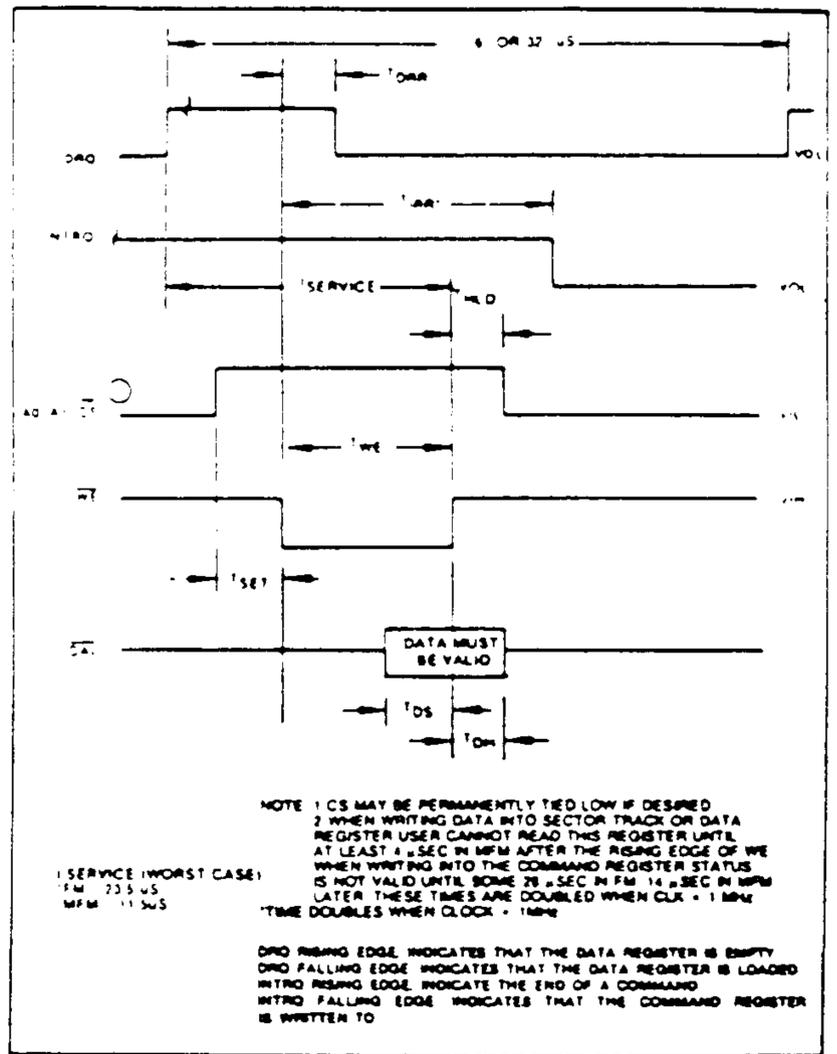
FIGURE 4. WRITE ENABLE TIMING
