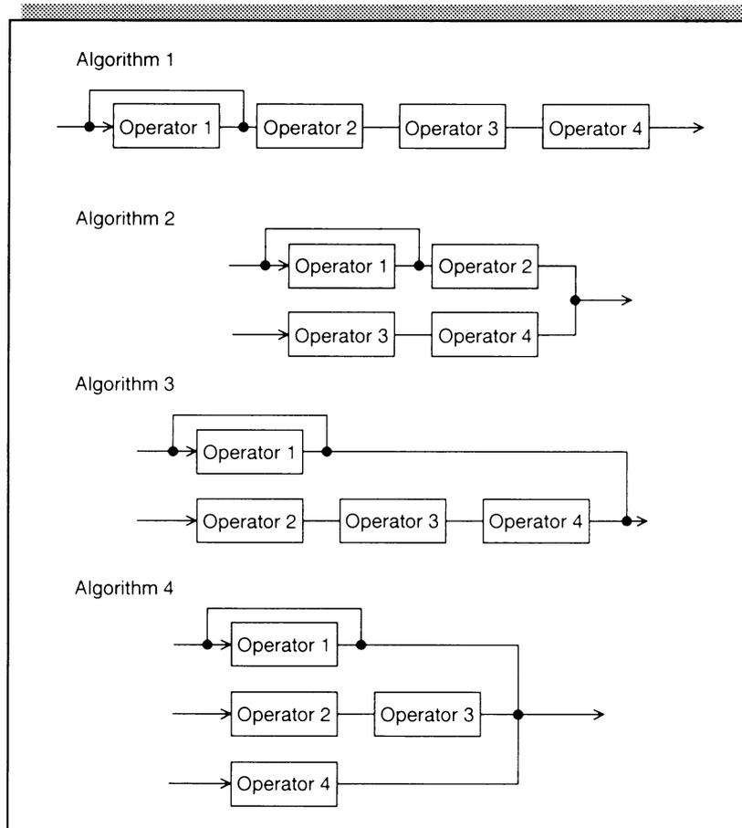
In the four-operator mode, the slot numbers corresponding to operators 1, 2, 3, and 4 are fixed, the same as in the two-operator mode.
