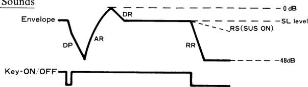
■ TIMING DIAGRAMS (Standard timing settings are V<sub>IH</sub> = 2.0V, V<sub>IL</sub> = 0.8V)
