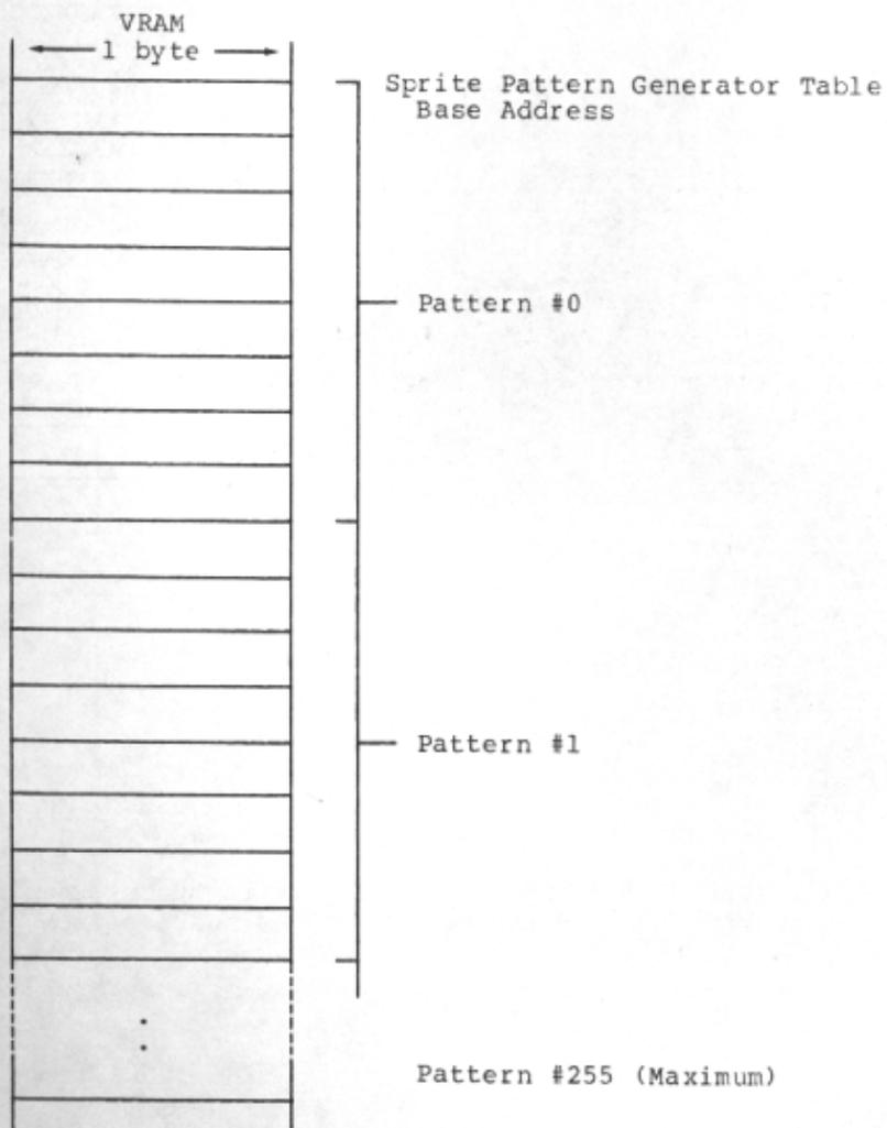
1.5 Example of Data Setting for Sprite Pattern Generator Table (G1, G2, MC)
