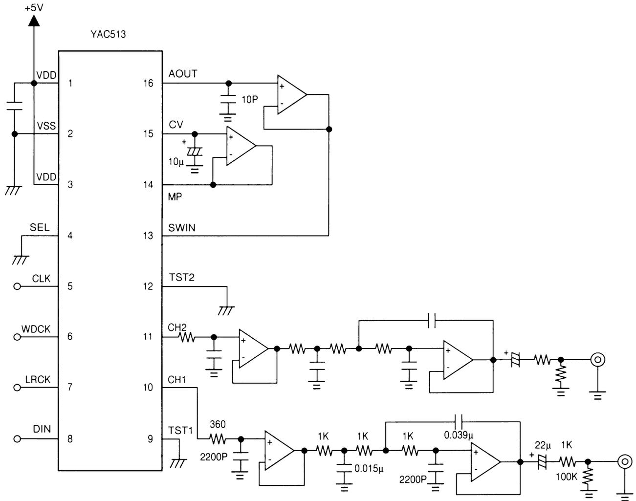
The CH1 and CH2 low-pass filters are the same circuit.
