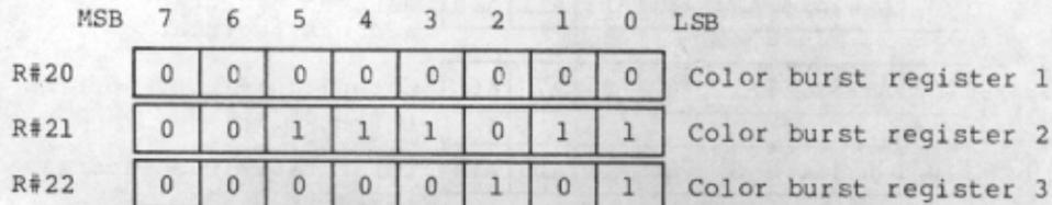
The above values are preset when the power is applied. If all values in the above three registers are set to 0, the color burst signal of the composite video output will be erased.
