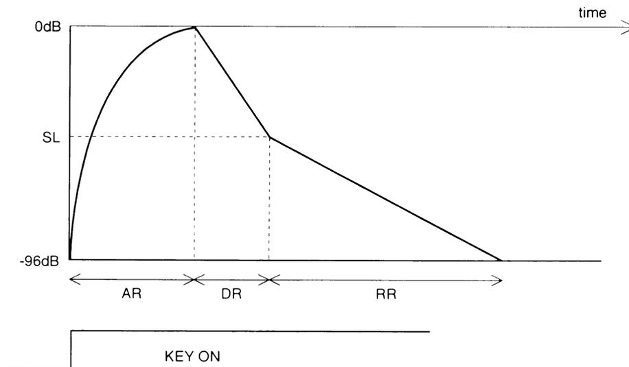
The attach rate changes exponentially with the time from key on to 0dB.
