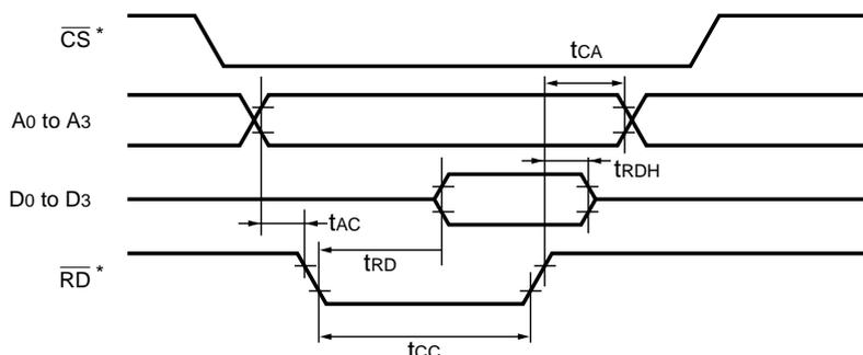
\*) The RP/RF5C01A accept  $\overline{RD}$  signals only when  $\overline{CS}="L"$  and  $CS="H"$  as in the case of  $\overline{WR}$  signals. Thus, substitute  $\overline{RD}$  signals shown above, as in the case of  $\overline{WR}$  signals, with  $\overline{CS} \cdot \overline{RD}$  signals to be applicable to the RP/RF5C01A configuration.
