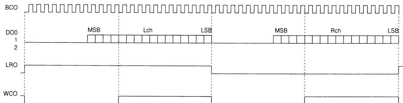
The BCO frequency is 48fs. Its duty is 50%. (fs=44.1kHz)
