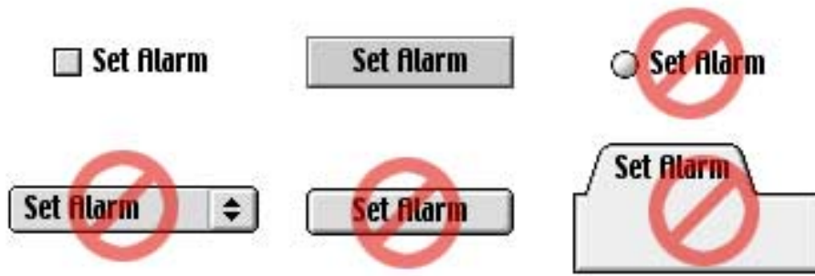
Figure 5. By allowing only certain controls to be used for a particular function, the Human Interface Guidelines can be enforced in a skinnable application. In this case, a checkbox and a "sticky" bevel button are appropriate, but a radio button, a popup menu, a pushbutton and a tab panel (!) are not.
