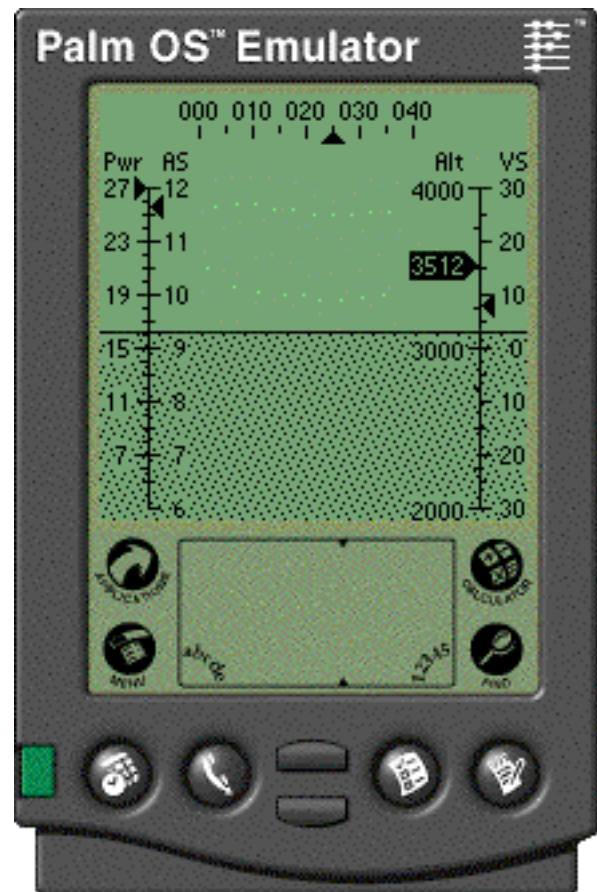
Figure 1. Integrated display view. Aircraft is in a wings-level climb.
