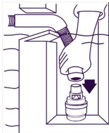
G: Place the New Kreepy Krauly into the pool and allow it to sink to the floor. Feed the hose down into the pool until it is completely filled with water. No air must be in the hose when it is fitted into the valve adaptor cuff.
