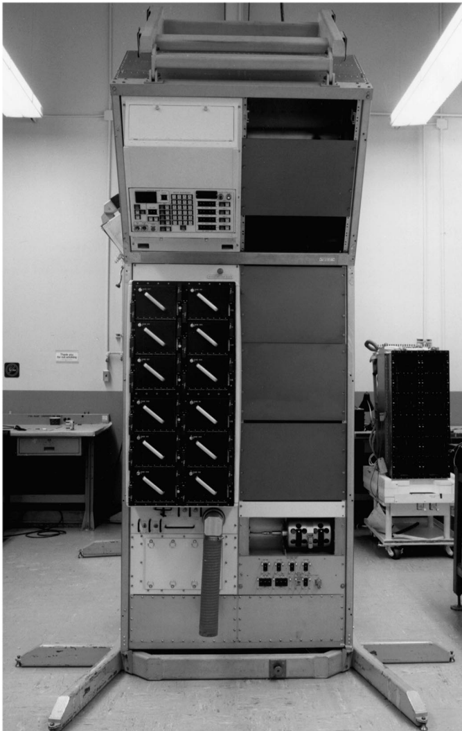
The rodent Research Animal Holding Facility is a self-contained unit providing food, water, temperature and airflow control, waste management and an automatic 12/12 light cycle for rodents used in life sciences research onboard the space shuttle.
